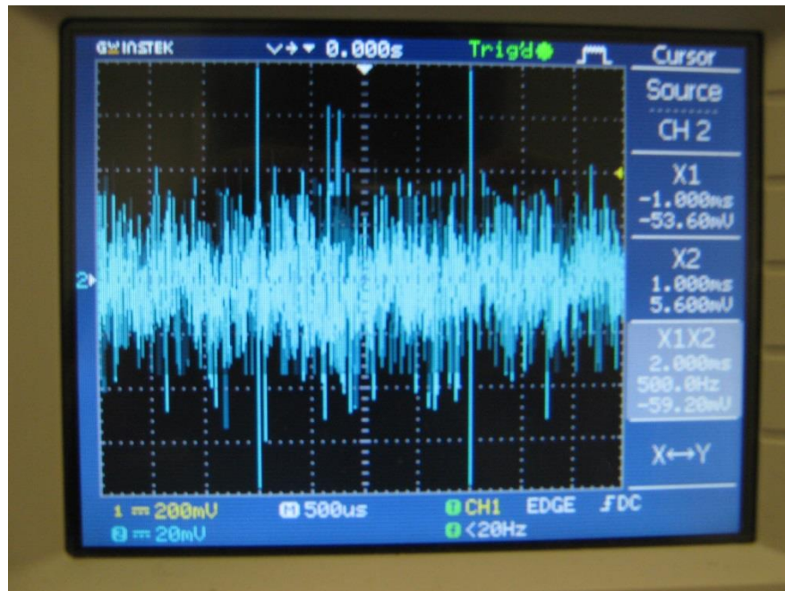
Figure 4.4: Graph of z-axis analog signal acceleration from accelerometer before applied low pass filter.
