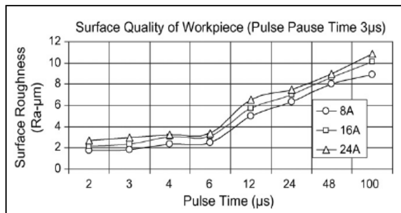
Figure 2.9: Effects of pulse time and pulsed current on surface roughness of workpiece (3 \mu s pulse pause time)
