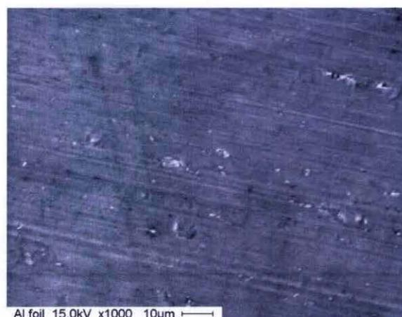
Figure 5.9 SEM image of Aluminum foil surface side for coating
