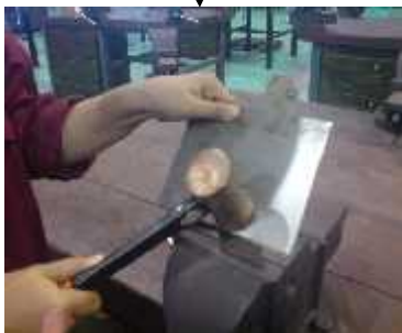
Bending process using hammer to bend the plate
