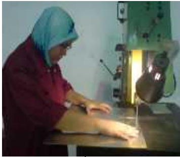
Cutting process using vertical bendsaw
