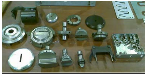
Figure 2.4: Accessories for Turret Punch Tool
