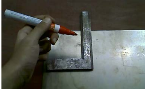
Figure 3.17: Marking Sheet Metal
