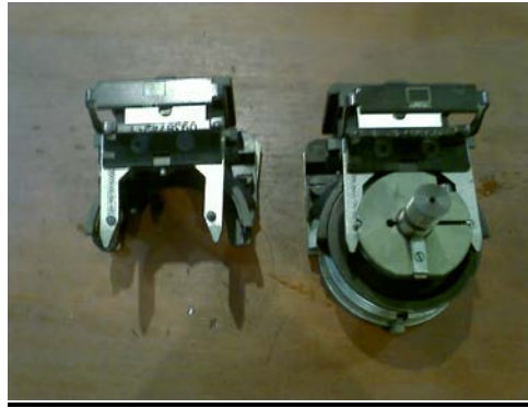
Figure 2.3: Main Tools of Turret Punch Machine; the Cartridge
