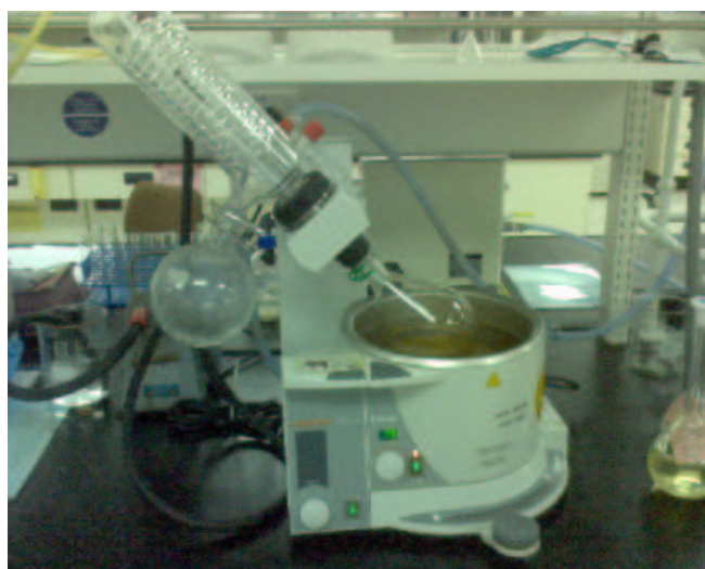
Appendix A.2: Rotary evaporator (Heidolph Laborata 4000 )
