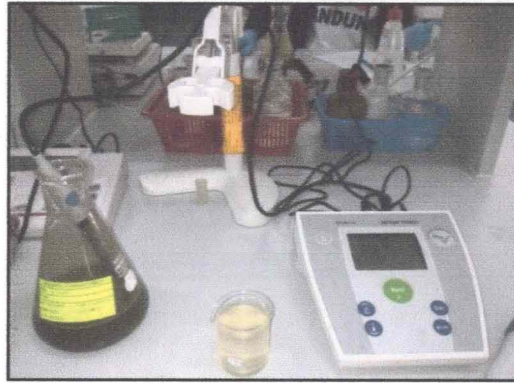
Figure 3.5 The electrode(s) of the pH meter was immersing into the water sample
