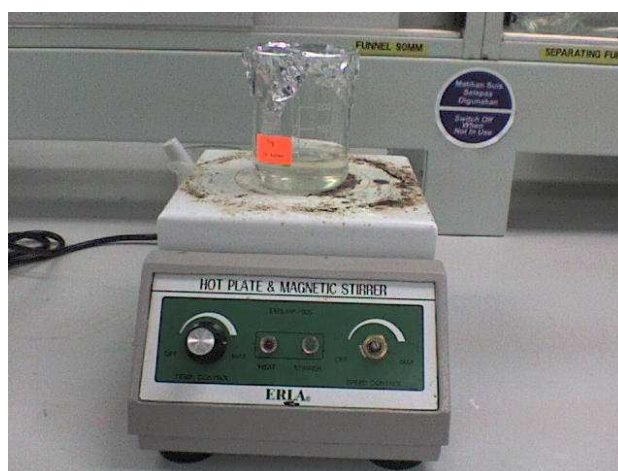
Figure 3.2: Preparation of dope solution using the hot plate and magnetic stirrer
