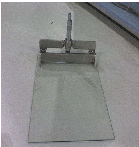
Figure 3.4 Casting flat sheet membrane using the casting knife
