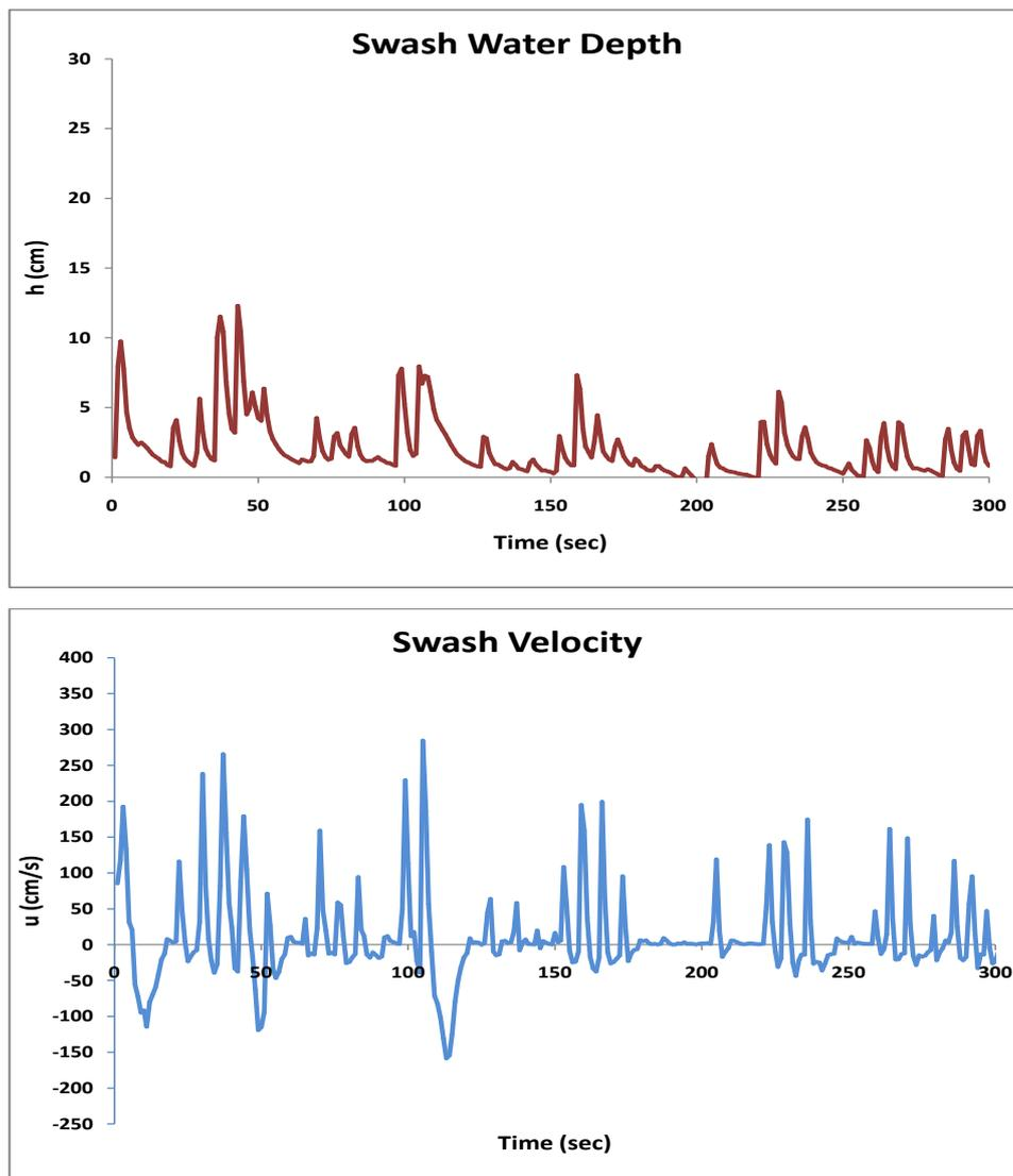
Figure 8. Profiles of swash water depth and velocity during dry season
