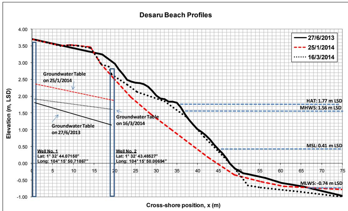
Figure 6. Beach profiles and mean groundwater level for 3 different days of monitoring
