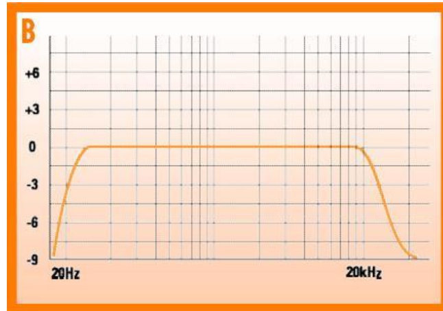
Figure 2.4: The desired Frequency Response
