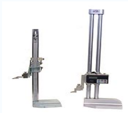
Figure 2.2: The left height gauge has the vernier scale, while the right one is an electronic height gauge with a digital readout.
