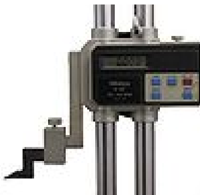
Figure 2.5: Electronic height gauge, close up view
