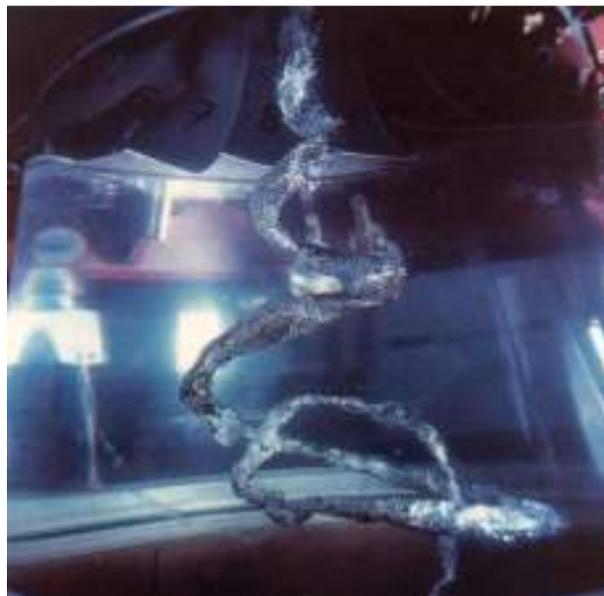
**Figure 2.3:** Example of cavitations in Francis Turbine
