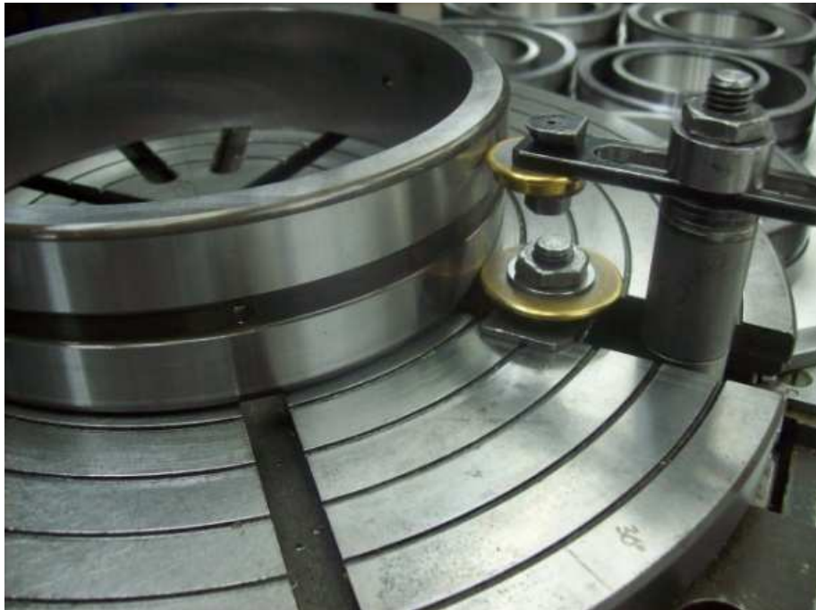
Figure 4 : Measuring device front tip. Operator must make sure correct fitting of the ring with the tip.
