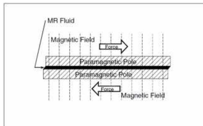
**Figure 1.2 :** MR fluid used in shear mode. [James. P ,2001]
