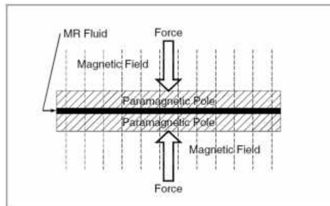
**Figure 1.1:** MR damper used in squeeze mode.[James. P ,2001]
