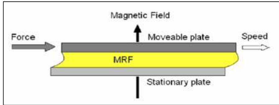
**Figure 2.1:** Shear mode. [Olabi A. G and Grunwald, 2007]
