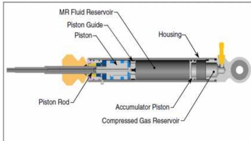
**Figure 2.5:** Mono tube MR damper section view.[ James. P, 2001]
