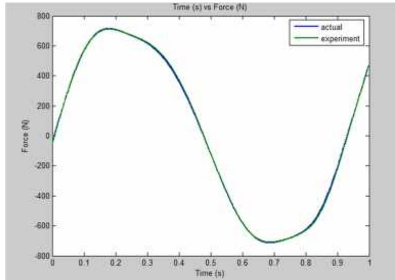
**Figure 4.24:** The comparison between actual (MR output) and experimental (NNSA output) graph for current 1.5A
