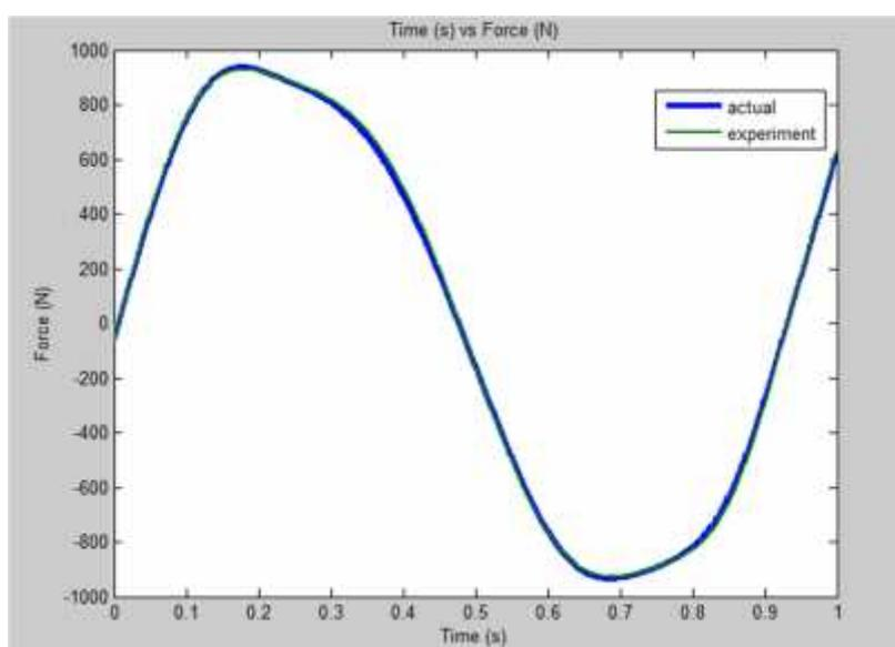
**Figure 4.28:** The comparison between actual (MR output) and experimental (NNSA output) graph for current 2A
