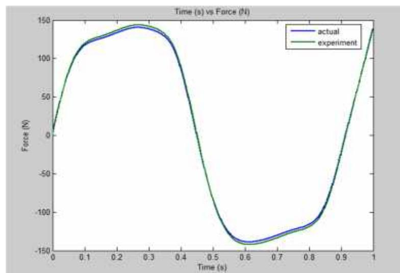
**Figure 4.12:** The comparison between actual (MR output) and experimental (NNSA output) graph for current 0A
