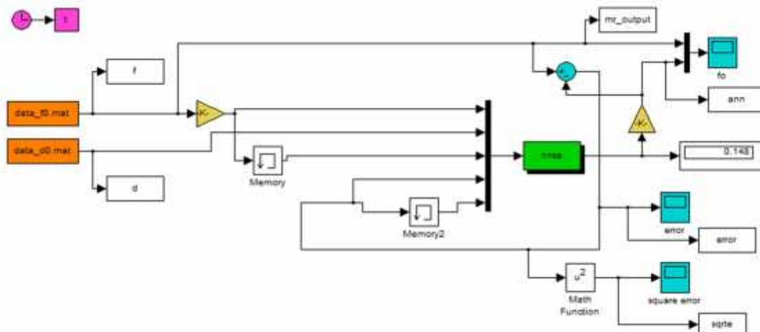
**Figure 4.1:** Simulink model
