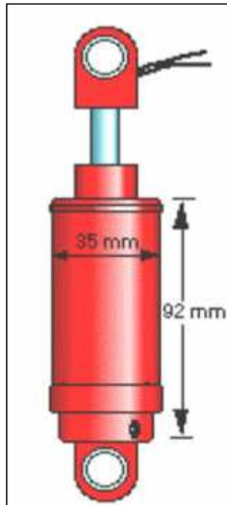
**Figure 2.4:** Magneto-rheological damper. [Schurter.K.C & Schurter. P. N.]
