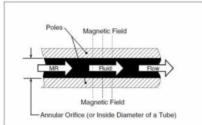
**Figure 1.3:** MR fluid used in valve mode. [James. P ,2001]
