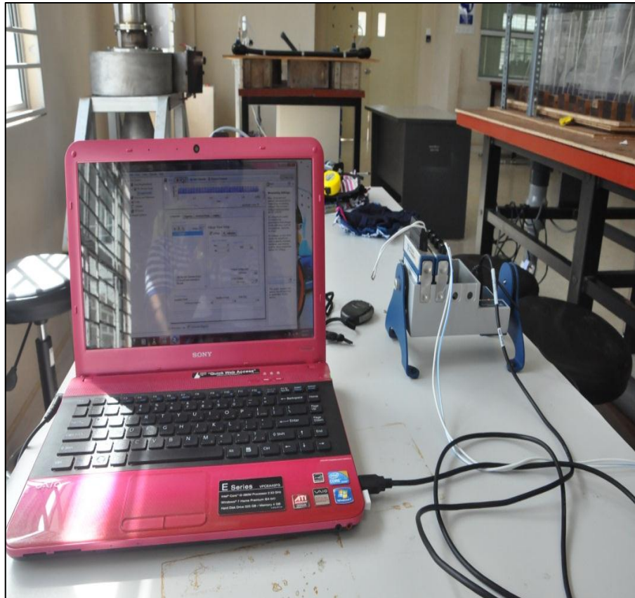
Figure 3.33: NI9239 is connected to the laptop
