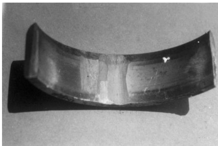
Figure 2.10: Defects on outer race of roller bearing
