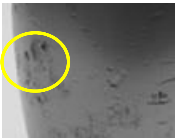
Figure 2.8: Hard particles caused contamination bruising on this roller bearing
