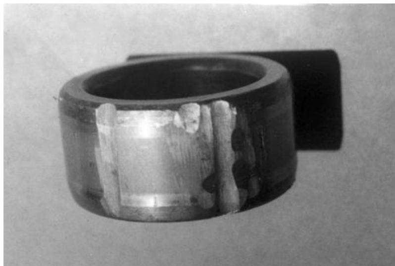
Figure 2.9: Defects on inner race of roller bearing
