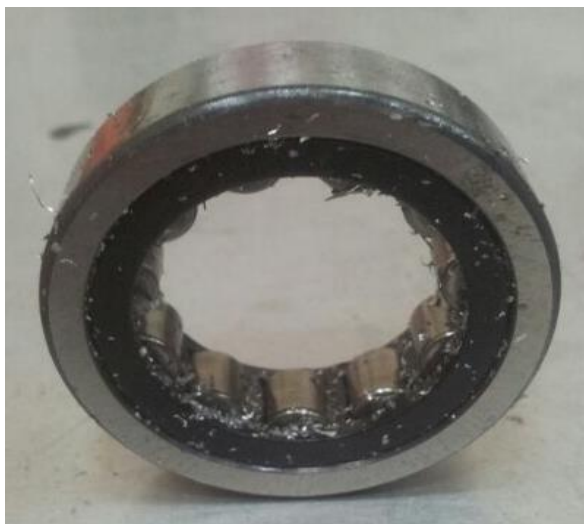
Figure 3.9: Contaminated defect bearing specimen
