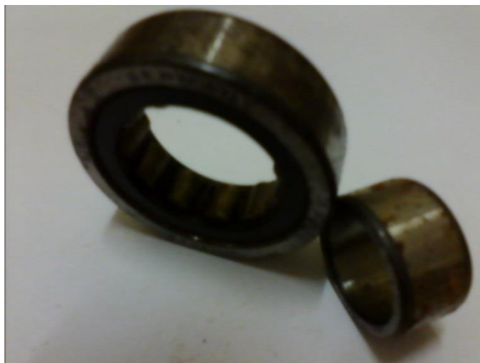
Figure 3.8: Corroded defect bearing specimen
