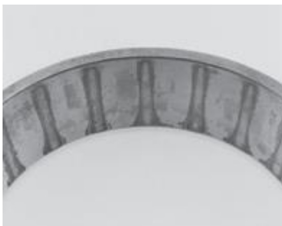
Figure 2.7: Heavy corrosion on the race
