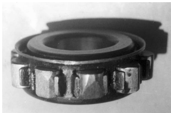
Figure 2.11: Defects on roller of roller bearing
