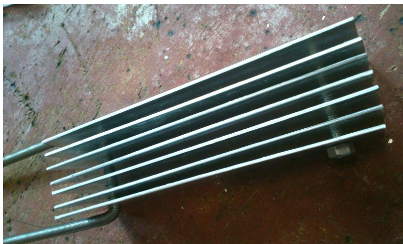
Figure 4.8: Stainless steel plate by stack in the hydrogen generator
