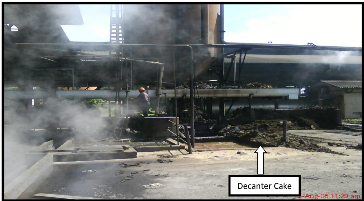
Figure 2.2: Decanter Cakes Produce from Lepar Hilir Palm Oil Milling Factory
