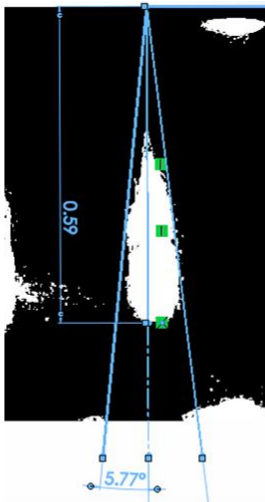
Figure 2.2: Definition of Spray angle and Spray tip Penetration
