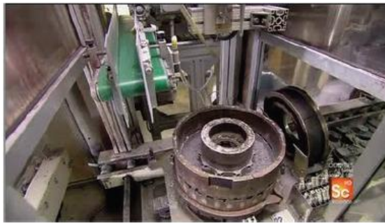
Figure 2.8: Permanent aluminum mold
