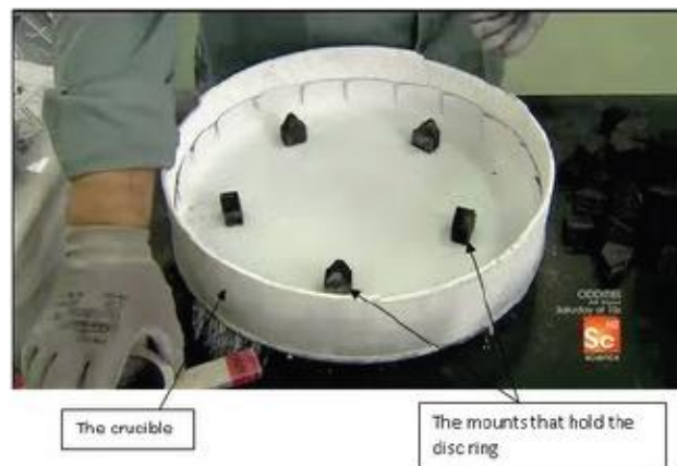
Figure 2.12: The crucible and the five mounts
