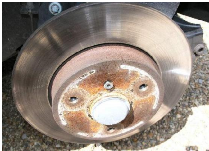
Figure 2.3: Example normal disc brake
