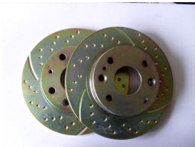
Figure 2.6: Example of combination disc brake
