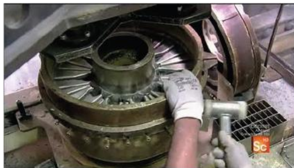
Figure 2.9: Mold setting process
