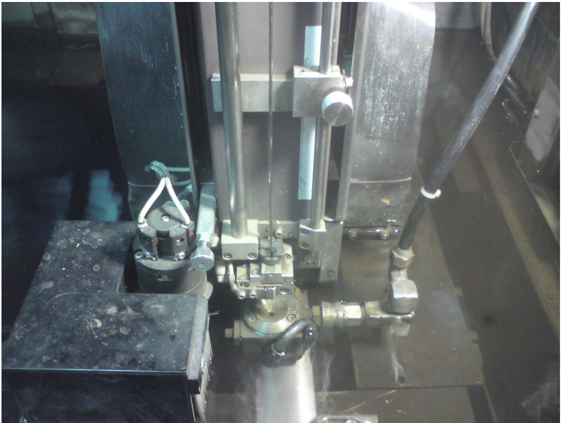
Wire cutting process in making precise crack on the cantilever beam.
