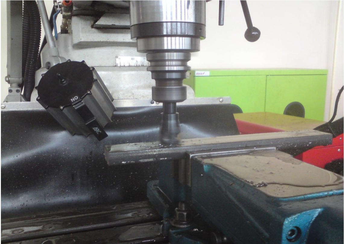
Milling process in fabrication of cantilever beam
