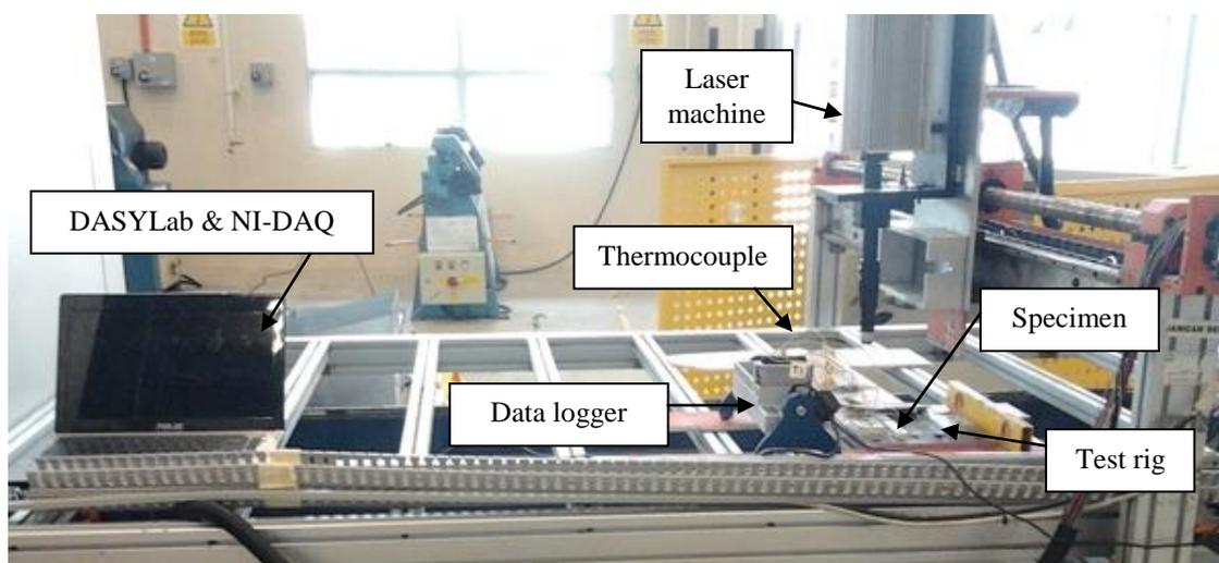
**Figure 3.11:** Experimental apparatus
