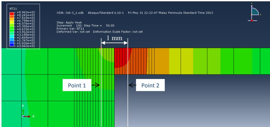
(a) Heating position at 50 % (3 mm) and 50 % (1 mm) with  $54 \times 10^6 \text{ W/m}^2$  of heat flux
