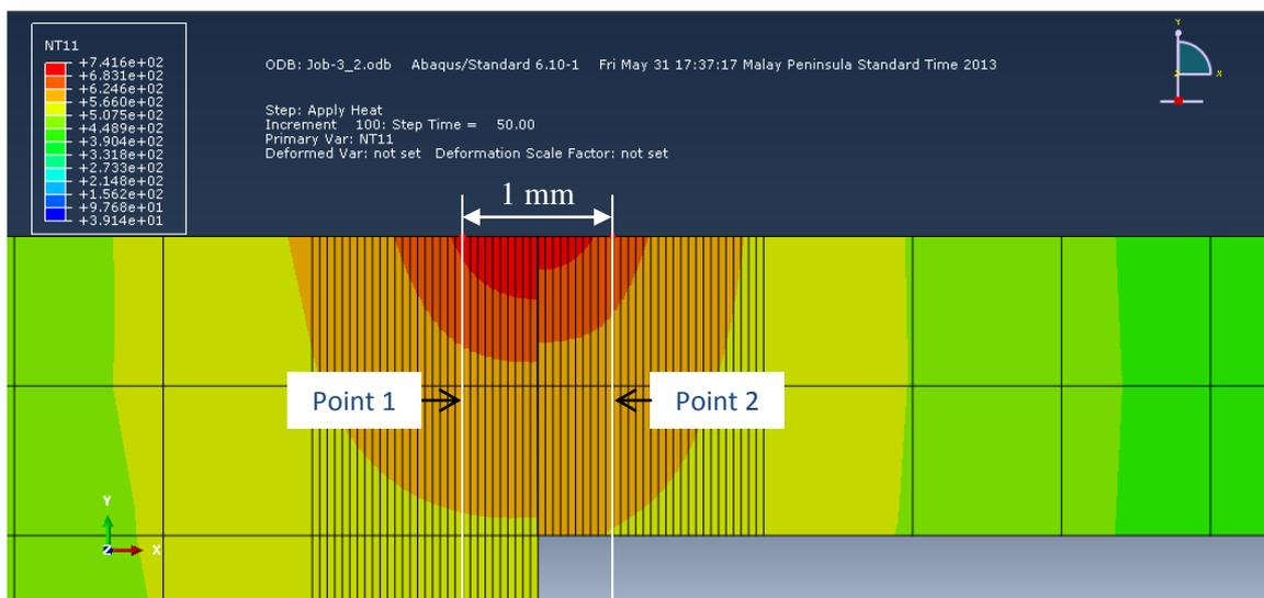
(b) Heating position at 55 % (3 mm) and 45 % (2 mm) with  $62 \times 10^6 \text{ W/m}^2$  of heat flux
