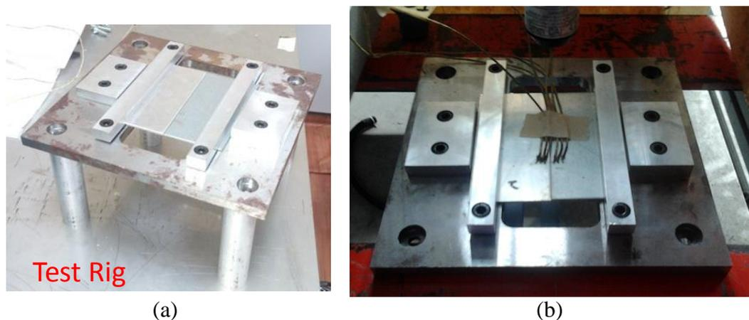
**Figure 4.1:** (a) Test rig, (b) Specimens material was clamped on the test rig
