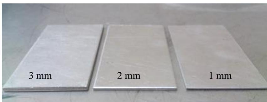
**Figure 3.7:** Specimen test (Aluminum 1100 material)
