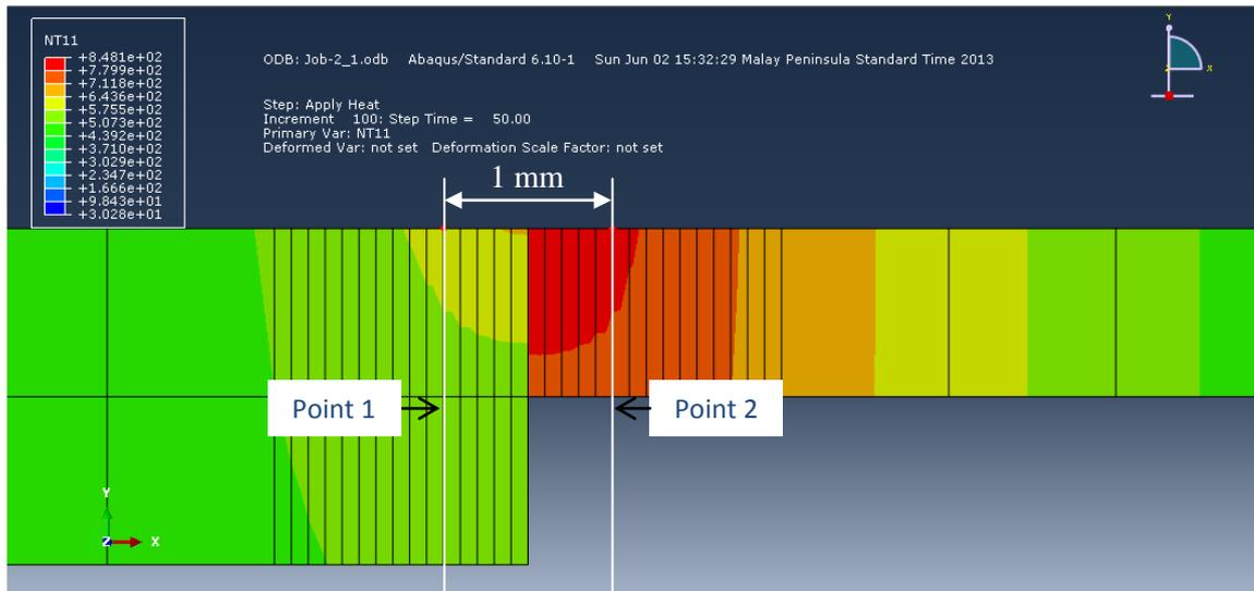
(a) Heating position at 50 % (2 mm) and 50 % (1 mm) with  $51 \times 10^6 \text{ W/m}^2$  of heat flux
