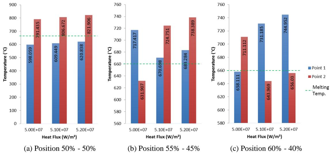
**Figure 4.7:** Temperature distribution for different position of heating and heat flux on thickness 2 mm with 1 mm
