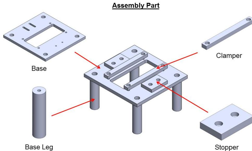
**Figure 3.3:** Assembly part of test rig
