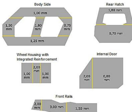
**Figure 2.2:** Typical parts made of tailored blanks
