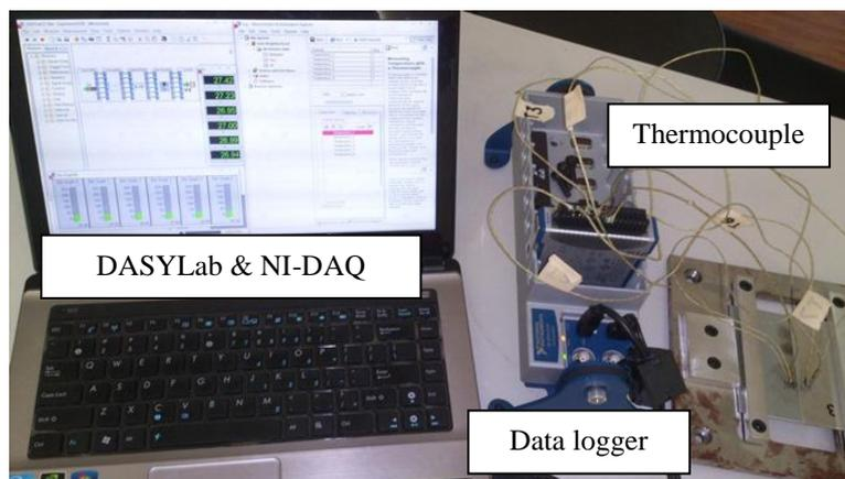
**Figure 3.10:** Measuring tools component
