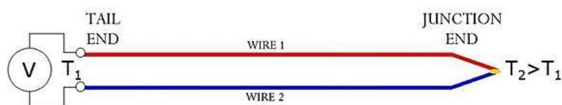
**Figure 2.8:** Schematic drawing of a thermocouple
