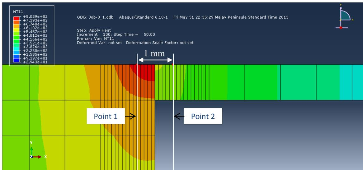
(c) Heating position at 70 % (3 mm) and 30 % (1 mm) with  $54 \times 10^6 \text{ W/m}^2$  of heat flux
