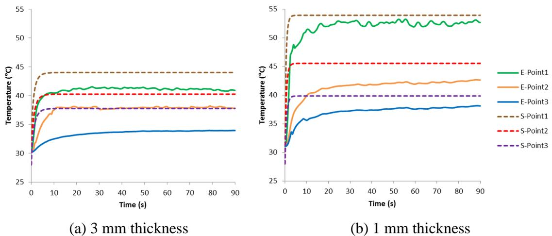
**Figure 4.2:** Comparison result for thickness 3 mm with 1 mm
