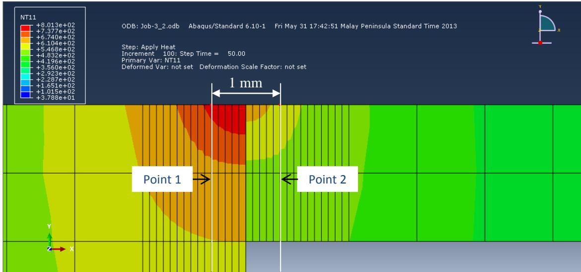
(c) Heating position at 60 % (3 mm) and 40 % (2 mm) with  $62 \times 10^6 \text{ W/m}^2$  of heat flux
