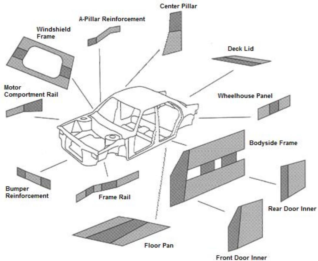
**Figure 2.1:** Exploded view of current and potential automotive tailor welded blank applications
