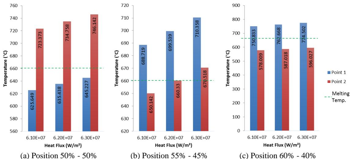
**Figure 4.6:** Temperature distribution for different position of heating and heat flux on thickness 3 mm with 2 mm
