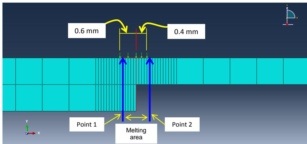
**Figure 3.13:** Position of heat imposed on modeling specimen for parametric study
