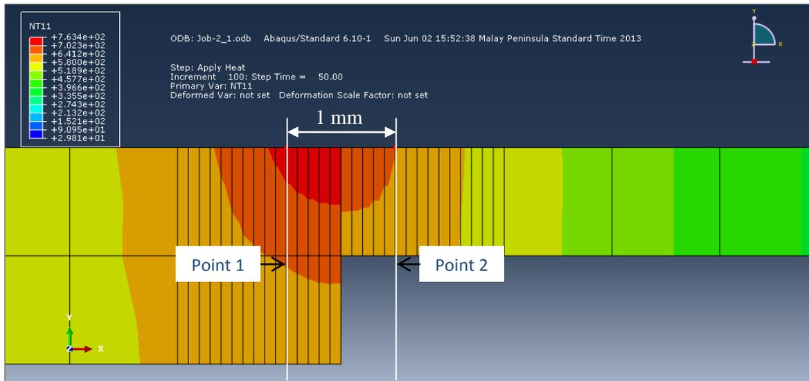
(c) Heating position at 60 % (2 mm) and 40 % (1 mm) with  $51 \times 10^6 \text{ W/m}^2$  of heat flux
