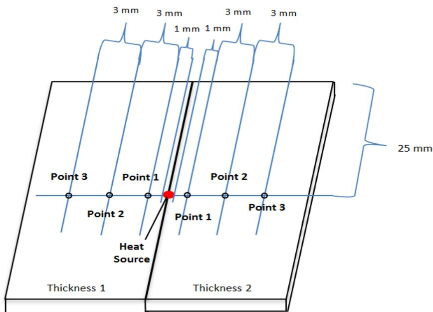
**Figure 3.9:** Position of points on the specimen
