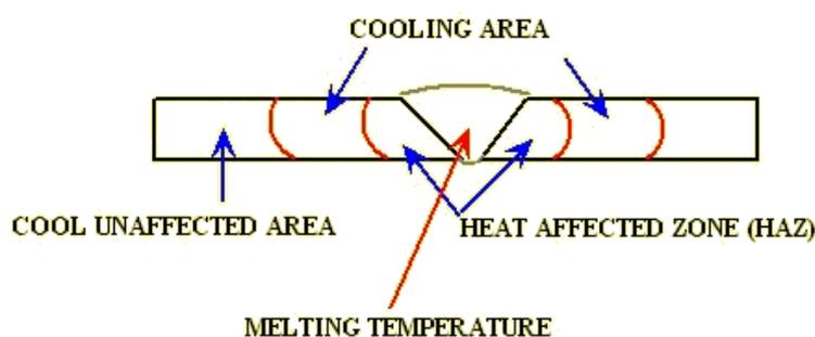
**Figure 2.7:** Schematic of heat affected zone
