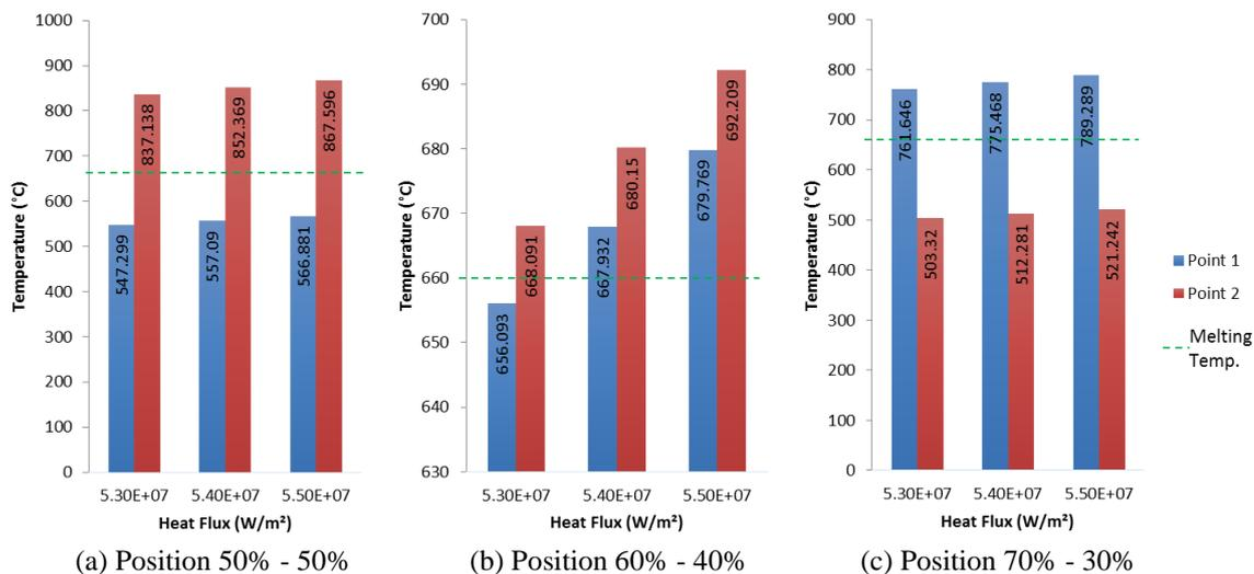
**Figure 4.5:** Temperature distribution for different position of heating and heat flux on thickness 3 mm with 1 mm
