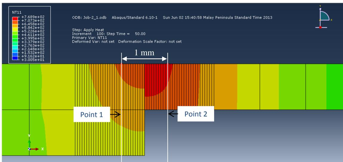
(b) Heating position at 55 % (2 mm) and 45 % (1 mm) with  $51 \times 10^6 \text{ W/m}^2$  of heat flux
