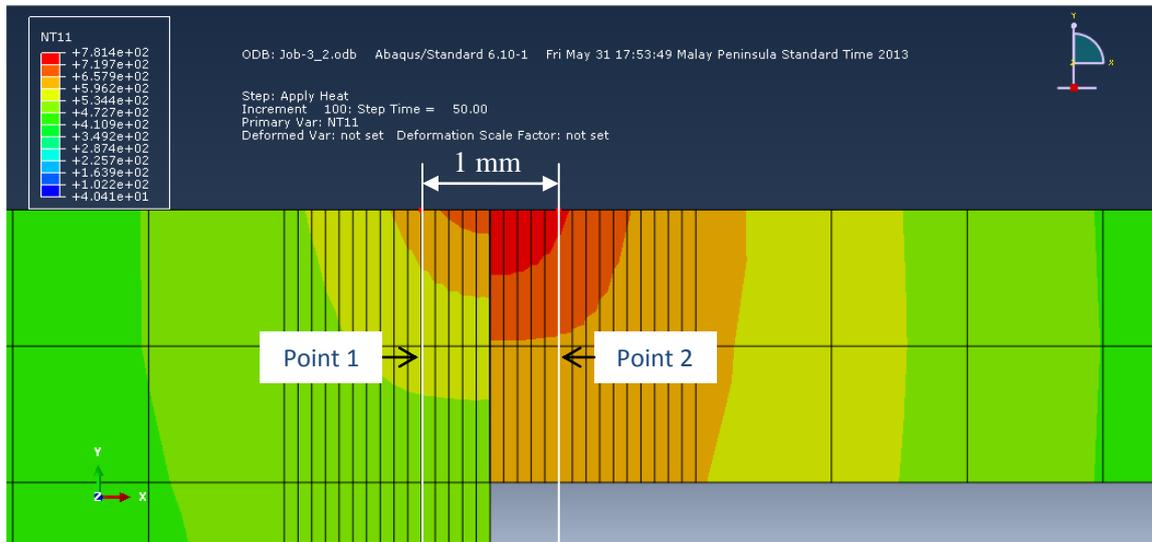
(a) Heating position at 50 % (3 mm) and 50 % (2 mm) with  $62 \times 10^6 \text{ W/m}^2$  of heat flux
