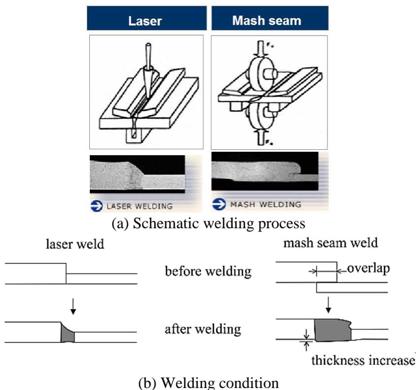
**Figure 2.5:** Laser and mesh seam welding
