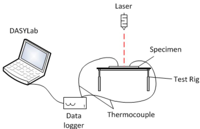
**Figure 3.6:** Schematic of experimental layout
