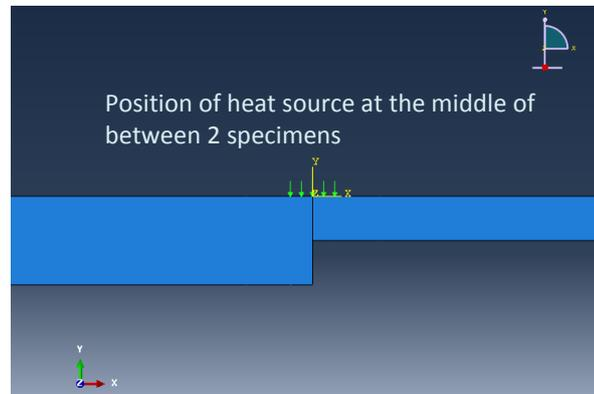
**Figure 3.12:** Position of heat source on specimen model for simulation
