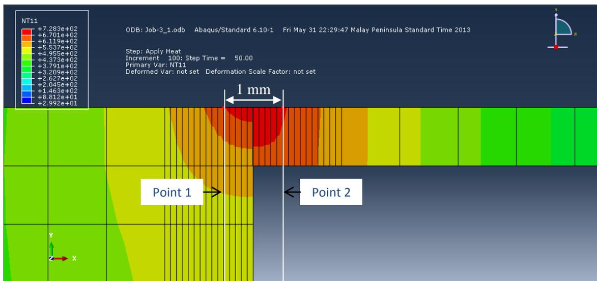
(b) Heating position at 60 % (3 mm) and 40 % (1 mm) with  $54 \times 10^6 \text{ W/m}^2$  of heat flux
