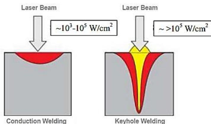
**Figure 2.6:** Comparison of conduction and keyhole welding
