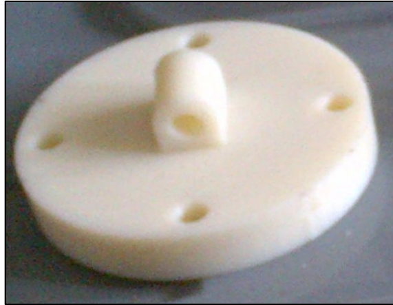
Figure 3.48: After supporting material removed
