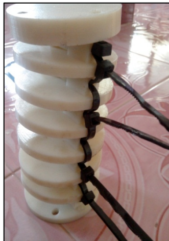
Figure 4.10: Cable tie replaced pin joint
