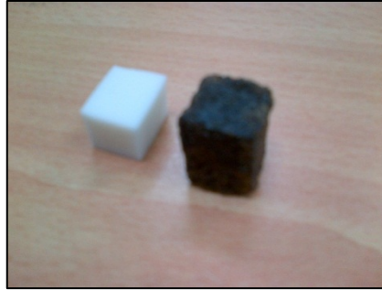
Figure 3.57: Rubber before compression test
