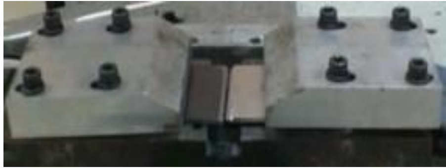
Figure 3.3: Structure was placed on the rig before welding.
