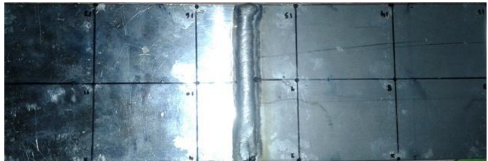
Figure 3.6: MIG weld structure that divided into 18 points.
