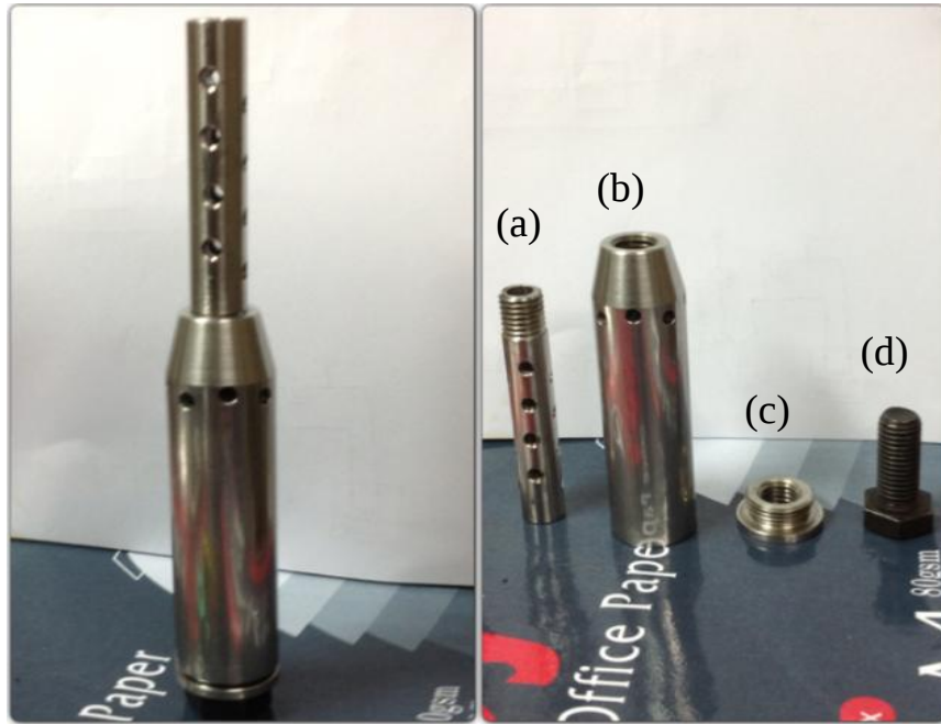
Figure 4.1: SST01 prototype igniter (Left), where a) Secondary chamber, b) Primary chamber, c) Bulkhead and d) Main igniter
