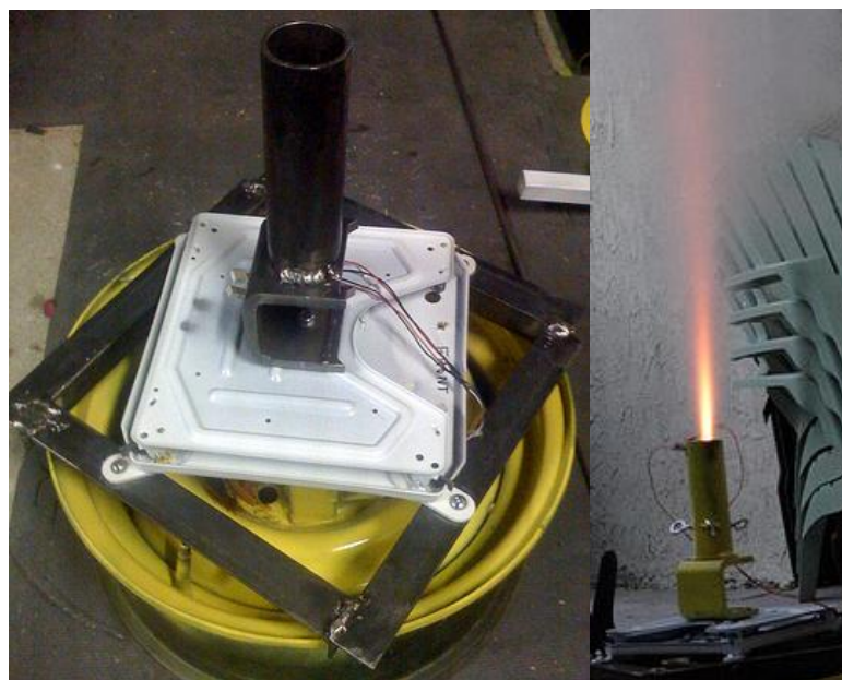
Figure 3.9: MK-1 strand burner model and testing cited from Examples of test strands for solid, liquid and hybrid rocket motor testing, http://aeroconsystems.com/cart/ts-pics
