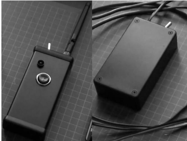
Figure 3.2: Transmitter (Left) and receiver (Right) for wireless ignition system
