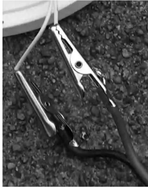
Figure 3.3: Connection between the igniter wire and alligator clips
