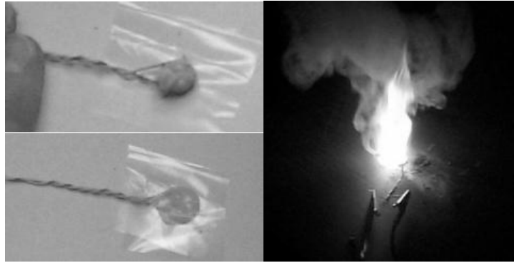
Figure 2.13: Ferocious igniter, where Top left: Pyrolant is applied onto poly sheet, Bottom left: Sealing of pyrolant by pressing it between two poly sheets and Right: Combusted Ferocious igniter
