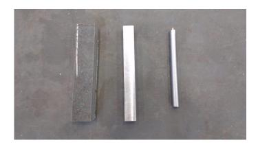
Figure 3.10: Transformation of raw material to specimen
