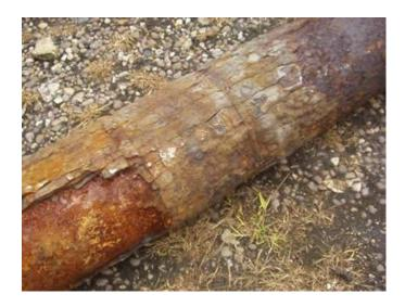
Figure 2.3: Corroded pipeline
