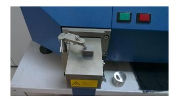
Figure 3.12: Optical emission spectrometry
