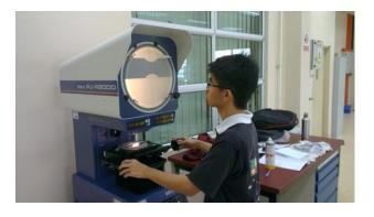
Figure 3.11: Profile projector to measure the notched dimension
