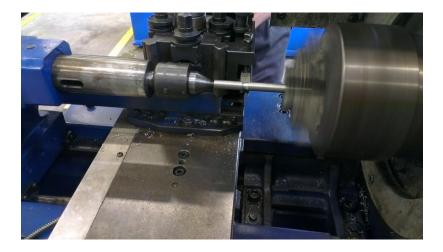
Figure 3.8: Turning process
