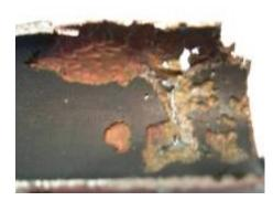
Figure 2.8: Erosion Corrosion
