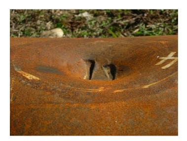
Figure 2.4: Defects of dents and gouges
