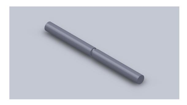
Figure 3.3: 1.5R notched tensile bar
