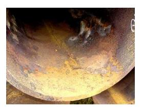
Figure 2.11: Internal corrosion
