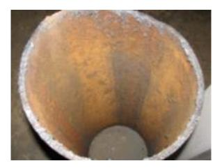
Figure 2.5: Generalized corrosion
