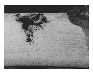
Figure 2.10: Intergranular corrosion
