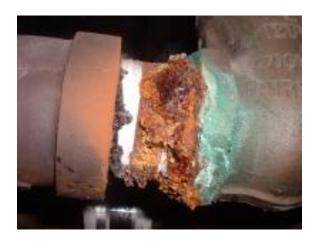
Figure 2.6: Galvanic corrosion
