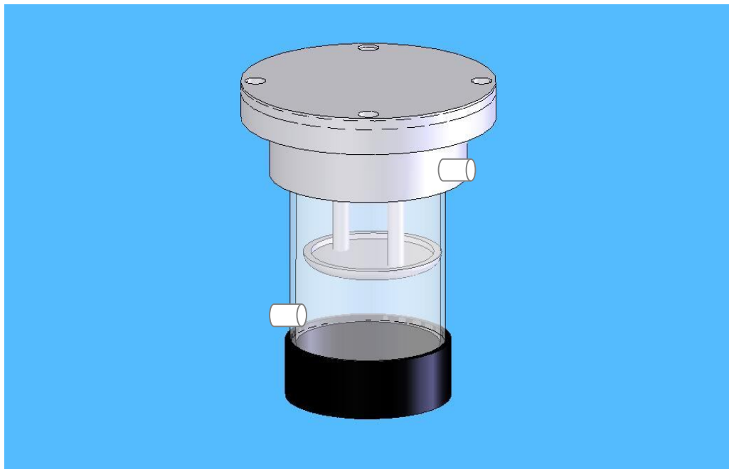
Figure 3.2: Solid Dessicant Dehydration Unit Design
