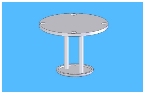
Figure 3.3 : Transparent plate with perforated tray
