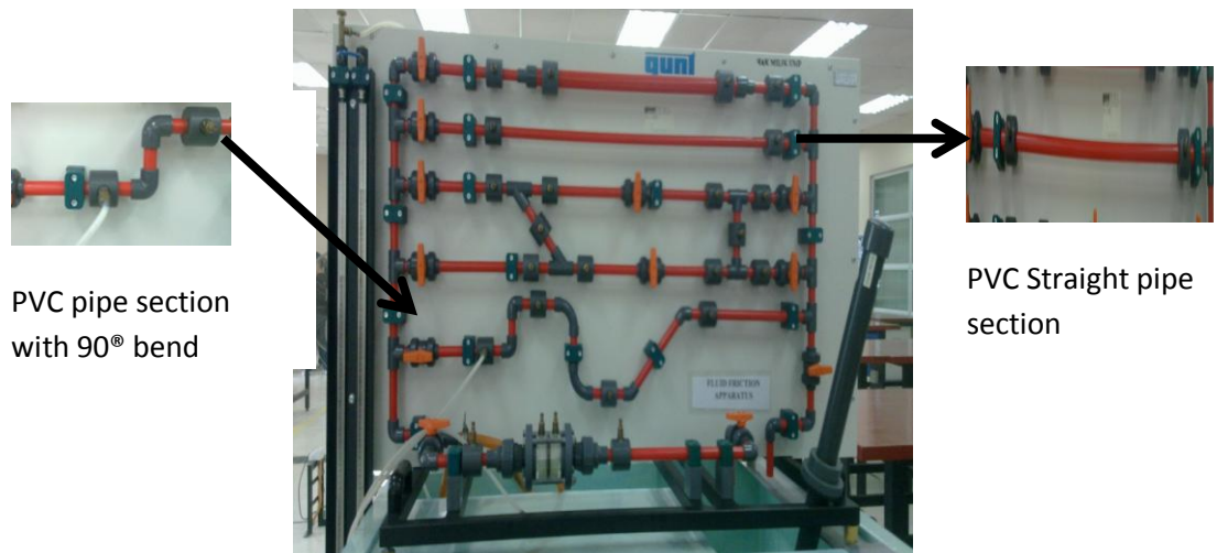
Figure 3.1: Fluid friction apparatus
