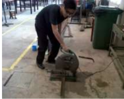
Figure 3.12: Cutting materials by using grinding machine
