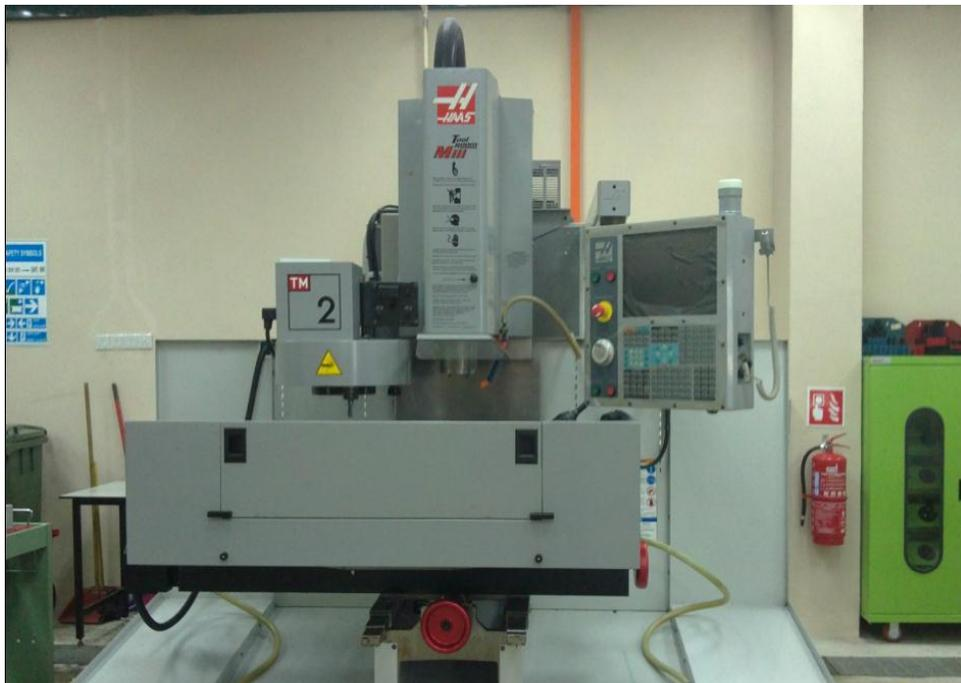
**Figure 3.2:** CNC milling machine model HAAS TM-2
