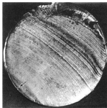
Figure 2.1: Sample of fatigue crack surface.
