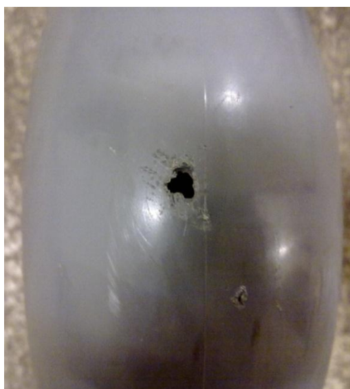
Figure 4.2 Cracked defected elbow
