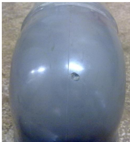
Figure 3.14 (2 mm) defect introduced on elbow
