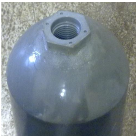
Figure 3.10 The PVC cap with socket connector
