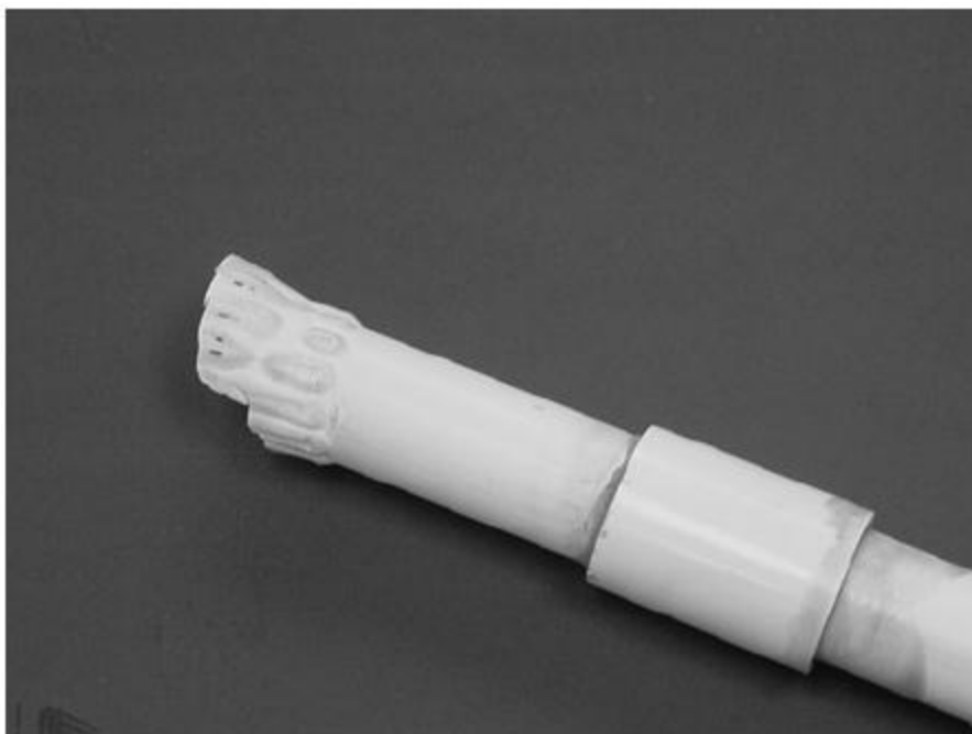
Figure 2.2 Softening failure of CPVC
