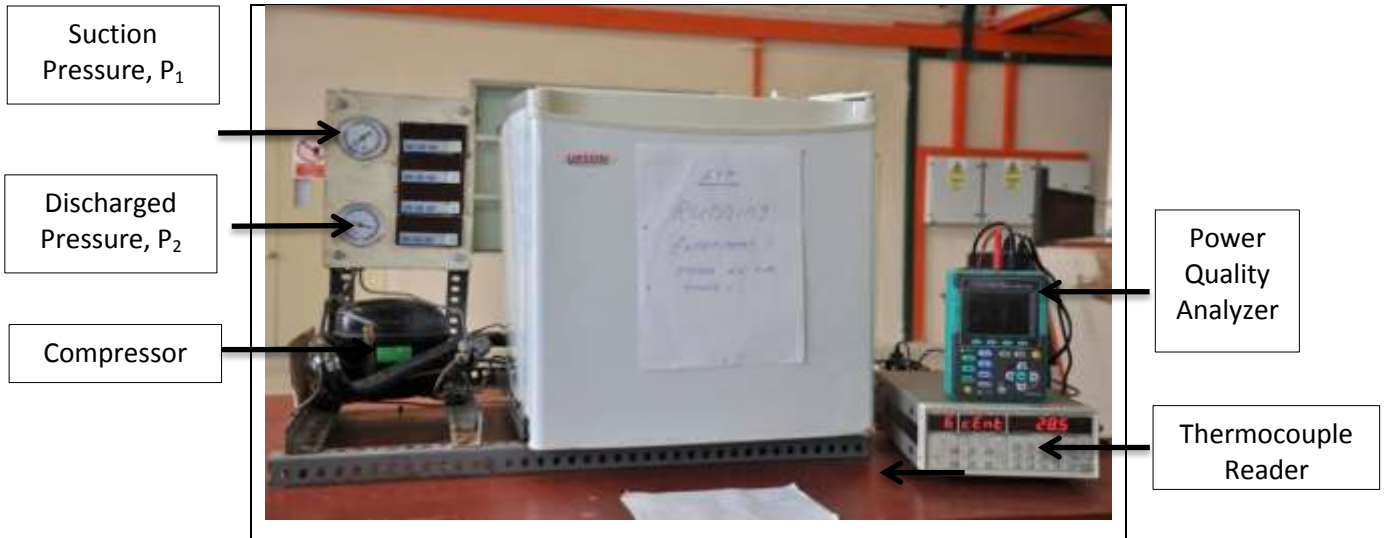
Figure 3.2: Experimental test rig of UPSON mini bar domestic refrigerator
