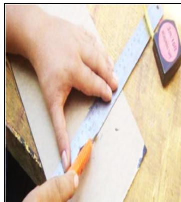
Figure 3.13: Measuring and marking process
