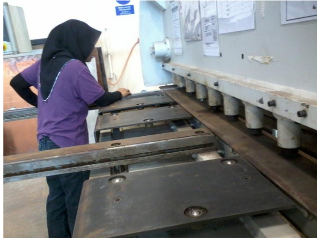
Figure 2.4 shows cutting process by using shear cutting machine
