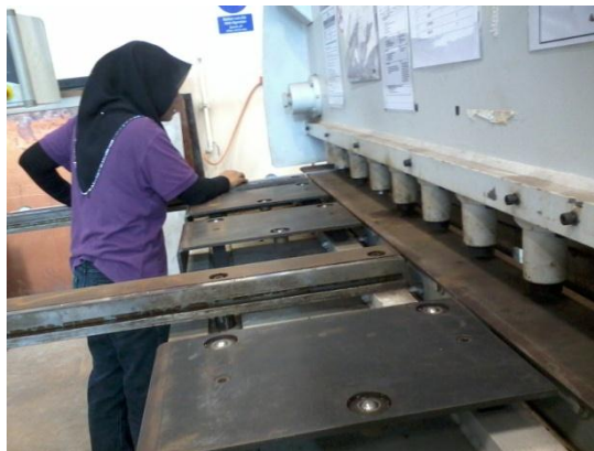
Figure 4.1 cut the aluminum plate by using shear cutting machine
