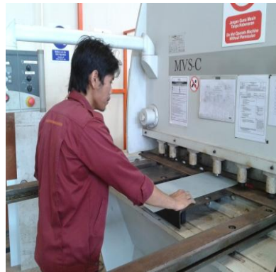
Figure 4.3: Cuts sheet metal using Cutting Machine
