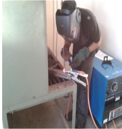
Figure 4.4: Welding the frame of the printer table
