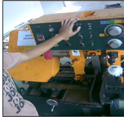
Figure 4.2: Cuts Materials using Bandsaw
