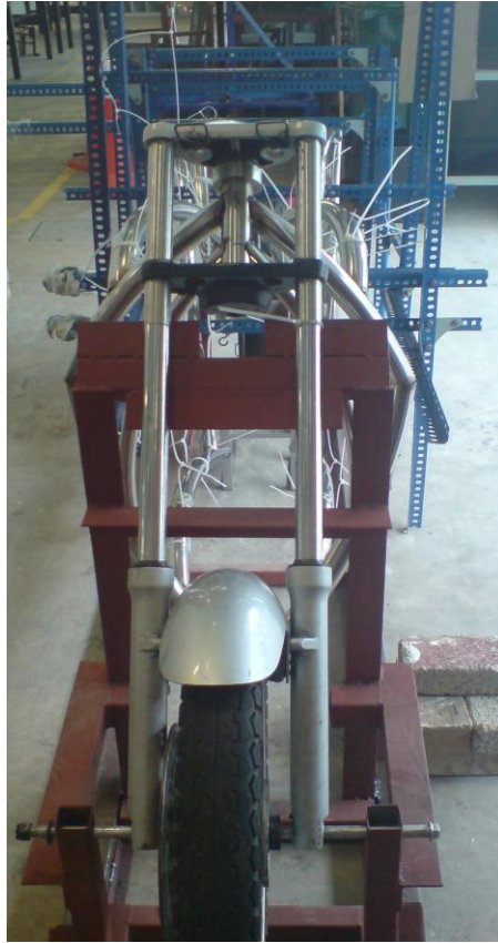
Figure 3.8 : Front suspension unit hold at rake 50 degree angle
