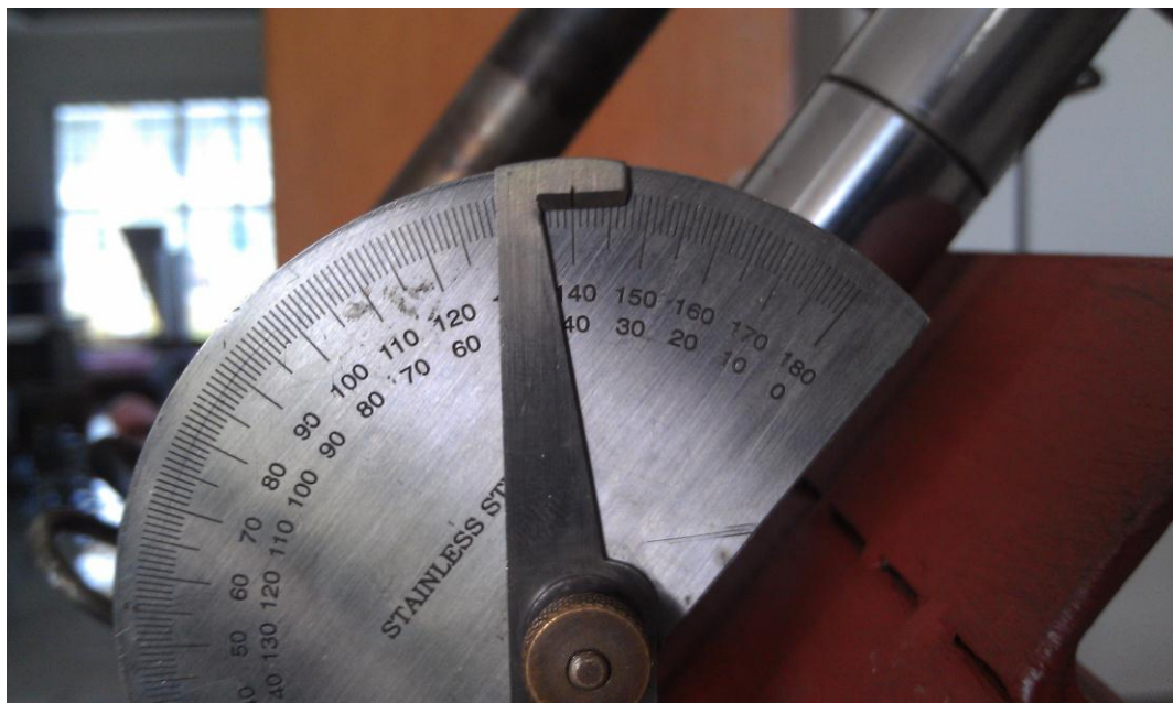
Figure 3.16 : 50 degree of slanted front suspension unit
