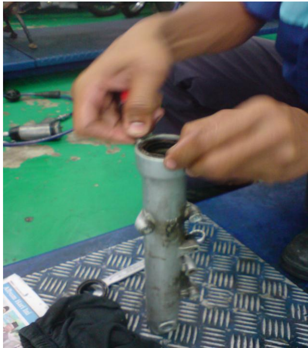
Figure 3.21 : Peel the O-ring from fork tube
