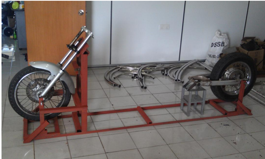
Figure 3.15 : A jig for front suspension 50 degree slanted
