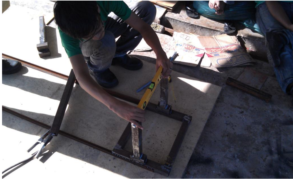
Figure 3.12 : Build the permanent front tyre holder at the jig
