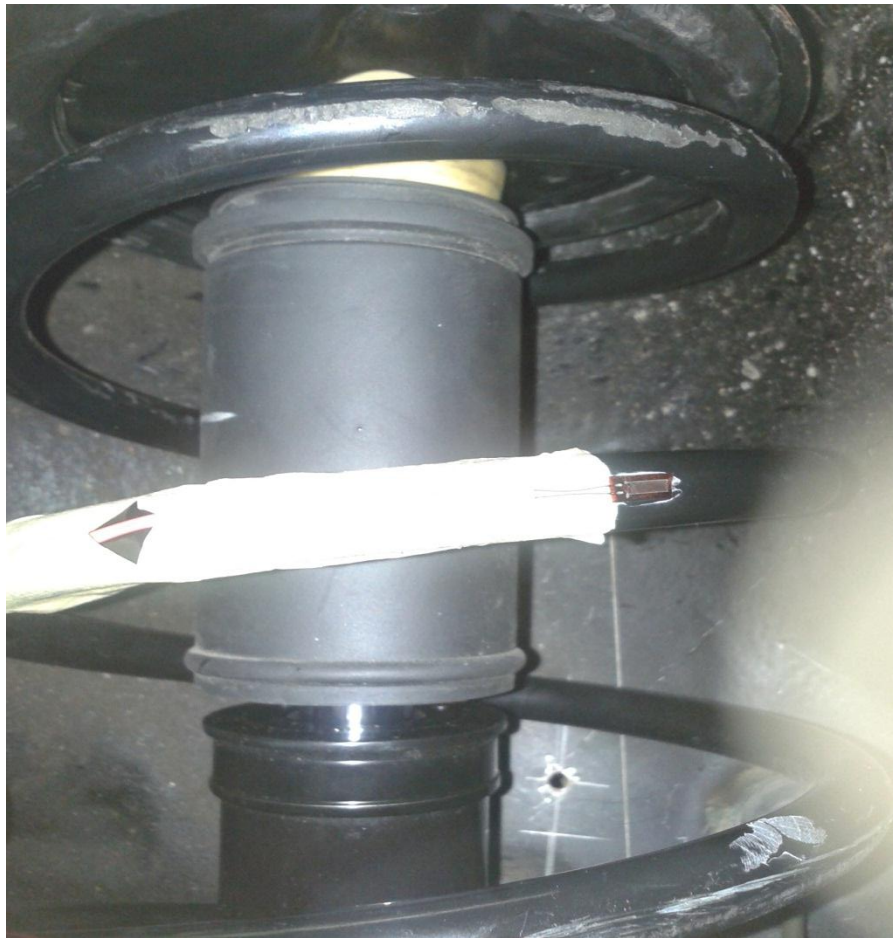
Figure 6.1: Strain gauge is glued on helical spring
