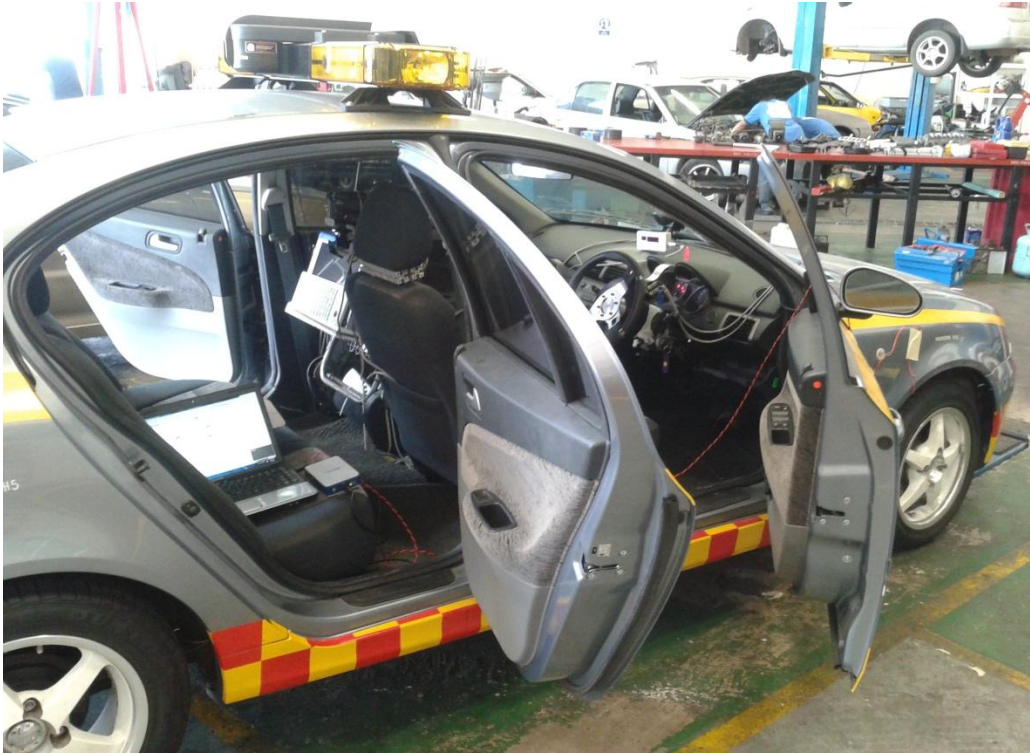
Figure 6.3: Setup of strain signal experiment at test car
