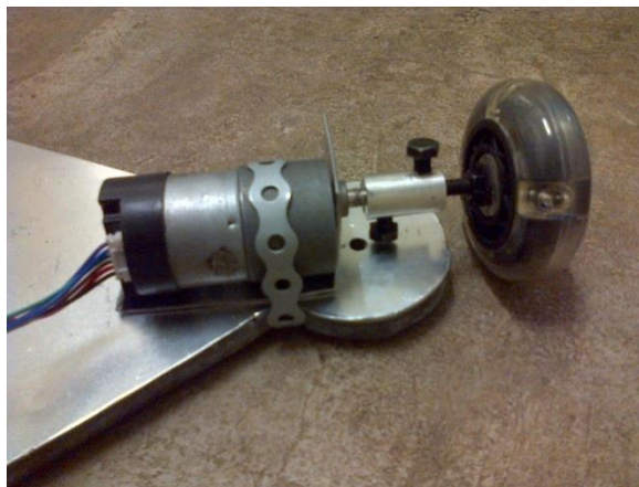
Figure 3.22: The motor that been attached to the platform
