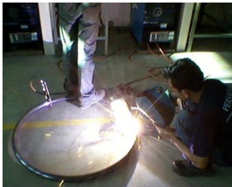
Figure 3.17: Welding Process Using MIG
