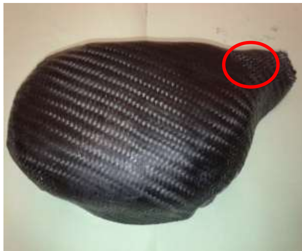
Figure 4.8 : The pattern of carbon fiber is change
