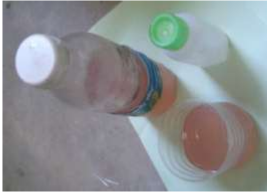
Figure 3.12 : Mixing the resin and hardener
