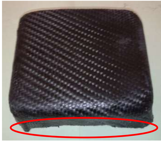
Figure 4.9 : The carbon fiber is not follow the shape of the part
