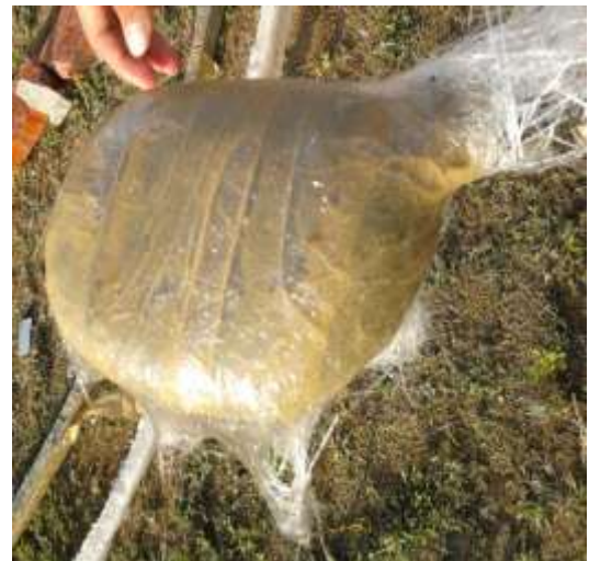
Figure 3.15 : Side mirror covered by glass fiber
