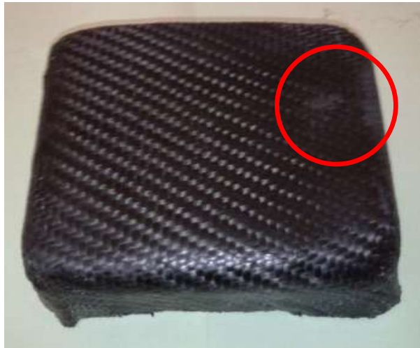
Figure 4.7 : Have a scratch on the surface
