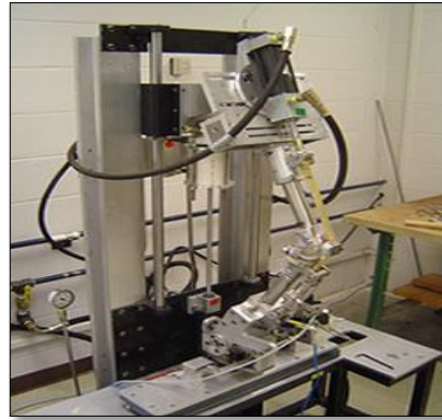
Figure 2.1: The Kansas knee simulator
