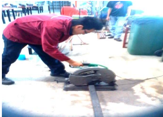
Figure 3.11: Cutting materials by using Cutting Machine
