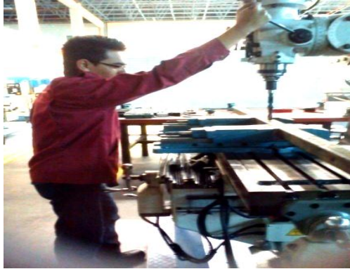
Figure 3.12: Drilling the holes by using Milling Machine
