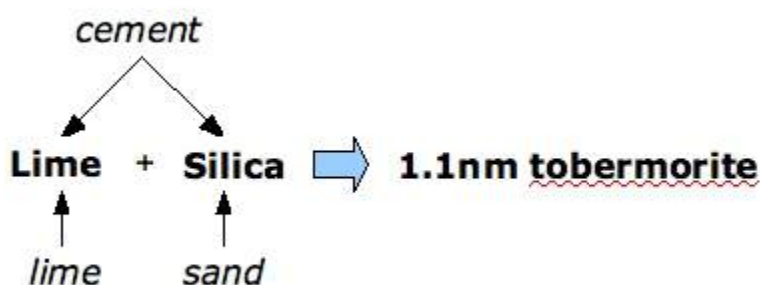
Figure 2.2.1: Chemistry notation of AAC composition
