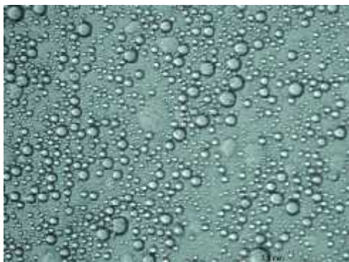
Figure 4.6: Photograph O/W emulsified biodiesel for 15 minutes mixing time.
