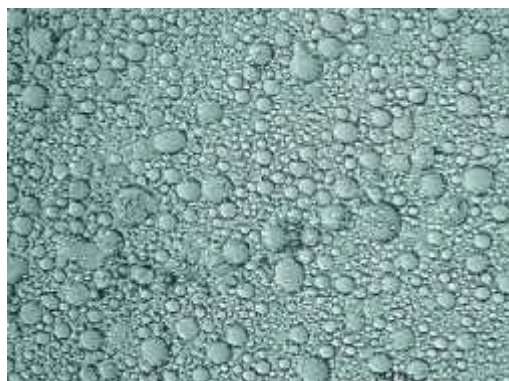
Figure 4.8: Photograph O/W emulsified biodiesel for 45 minutes mixing time.
