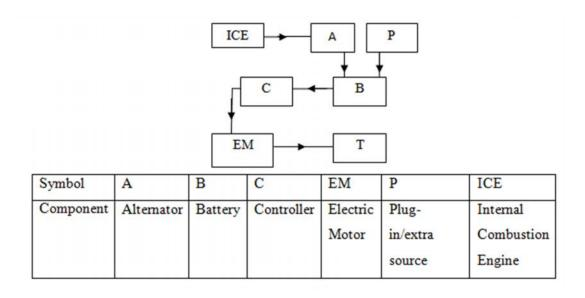
Figure 2.2: Series PHEM configuration
