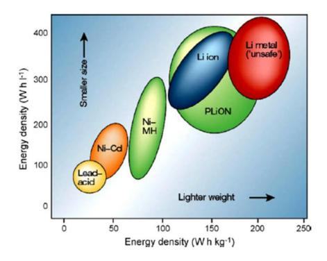
Figure 2.4: Volumetric energy density (Wh/L) with respect to gravimetric energy density (Wh/kg) for different variety of batteries
