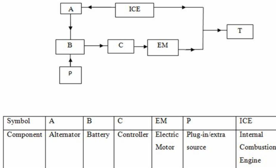
**Figure 2.3:** Parallel PHEM configuration
