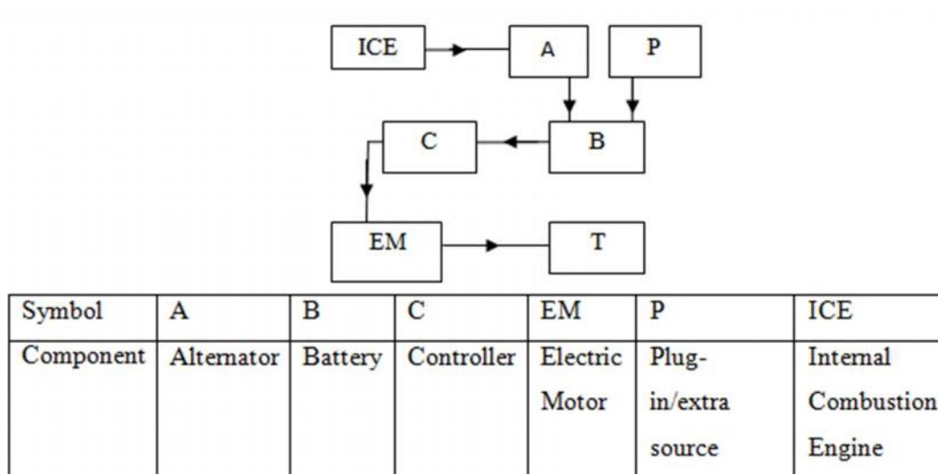
**Figure 2.2:** Series PHEM configuration
