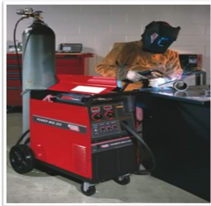
Figure 2.4: Metal Inert Gas (MIG) Welding
