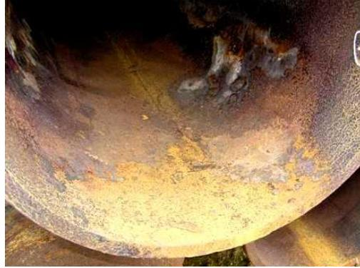
**Figure 2.11:** Internal corrosion
