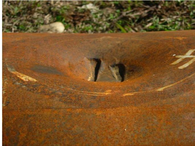
**Figure 2.4:** Defects of dents and gouges
