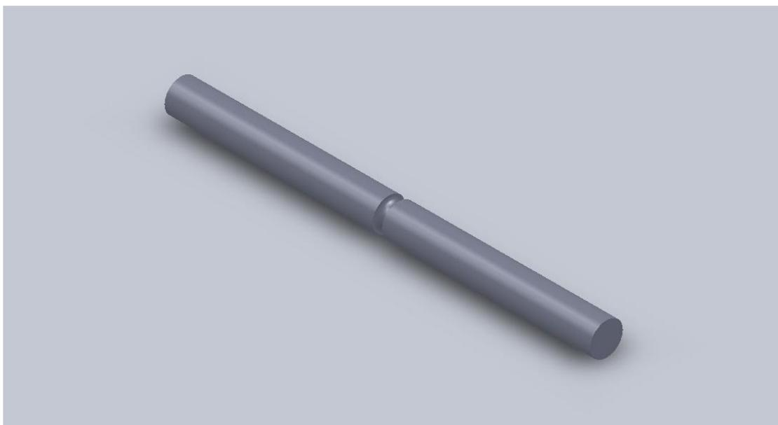
**Figure 3.3:** 1.5R notched tensile bar
