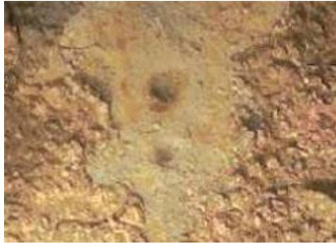
**Figure 2.7:** The rust indicates the pitting is occurring.
