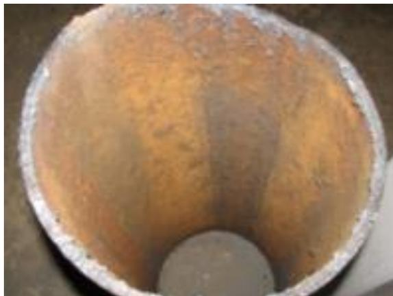
**Figure 2.5:** Generalized corrosion
