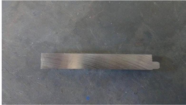
**Figure 3.9:** Tool, HSS create the notched part
