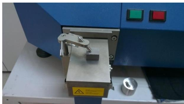
**Figure 3.12:** Optical emission spectrometry
