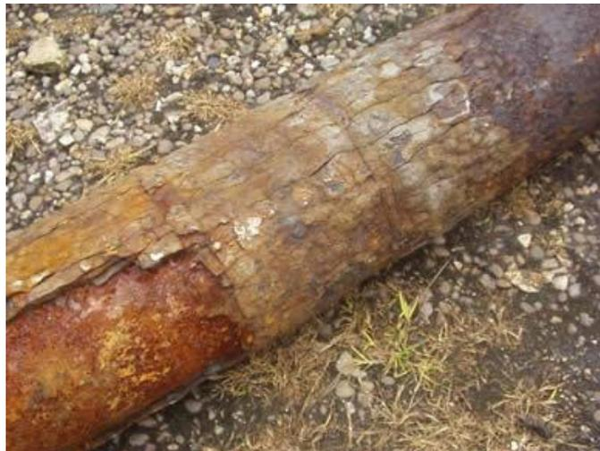
**Figure 2.3:** Corroded pipeline
