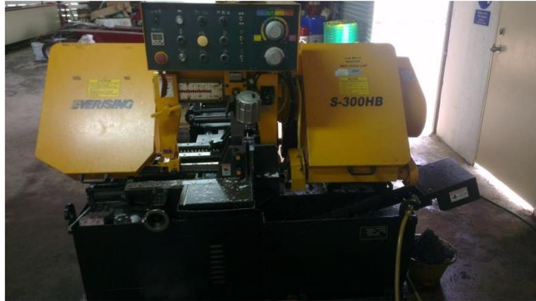
**Figure 3.6:** Hydraulic bend saw
