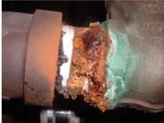
**Figure 2.6:** Galvanic corrosion
