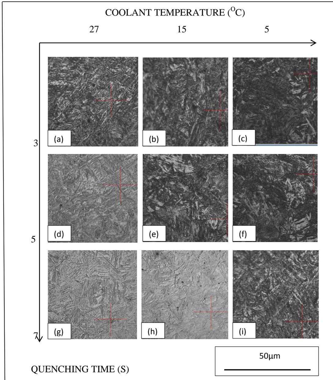
**Figure 4.7** Micrograph of martensite structure produced at different quenching time and coolant temperature of (a), (d), and (g)  $27^{\circ}\text{C}$ , (b), (e), and (h)  $15^{\circ}\text{C}$ , and (c), (f), and (i)  $5^{\circ}\text{C}$ .
