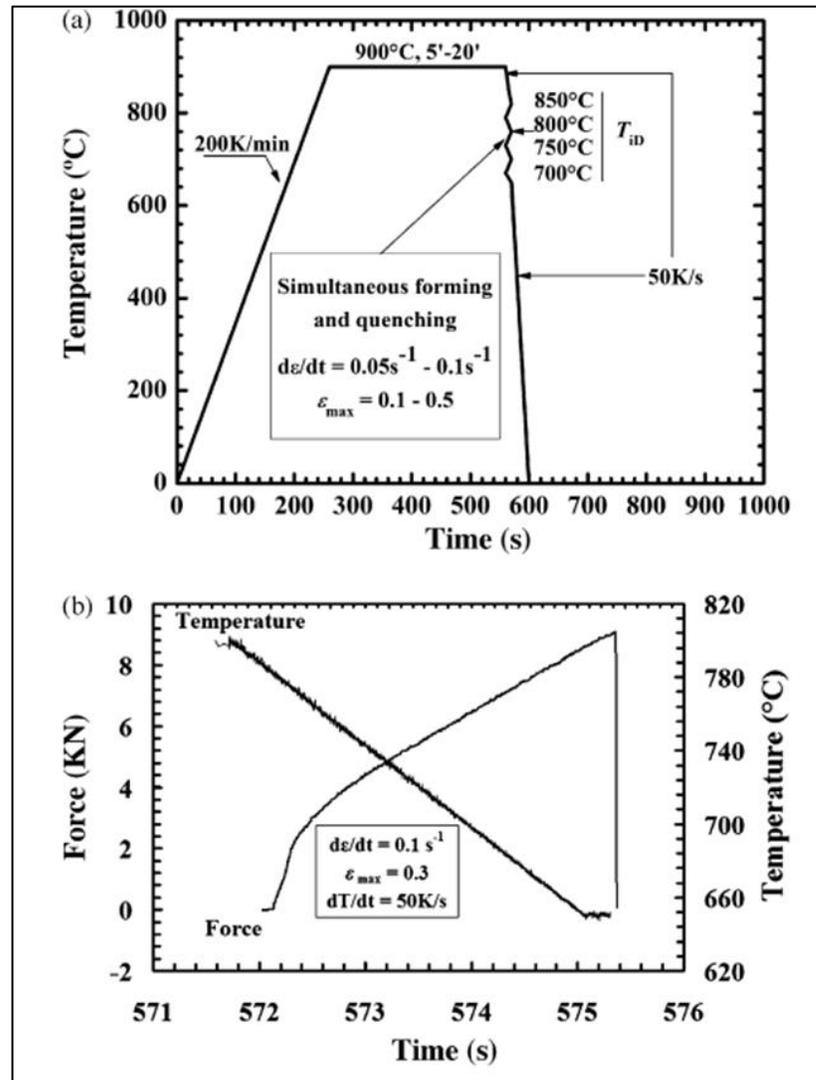
**Figure 2.4** The effect of applied force on phase transformations [11].
