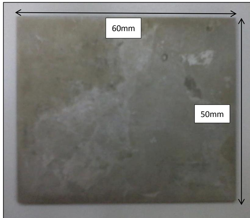
**Figure 3.2** Boron alloyed steel plate (22MnB5).
