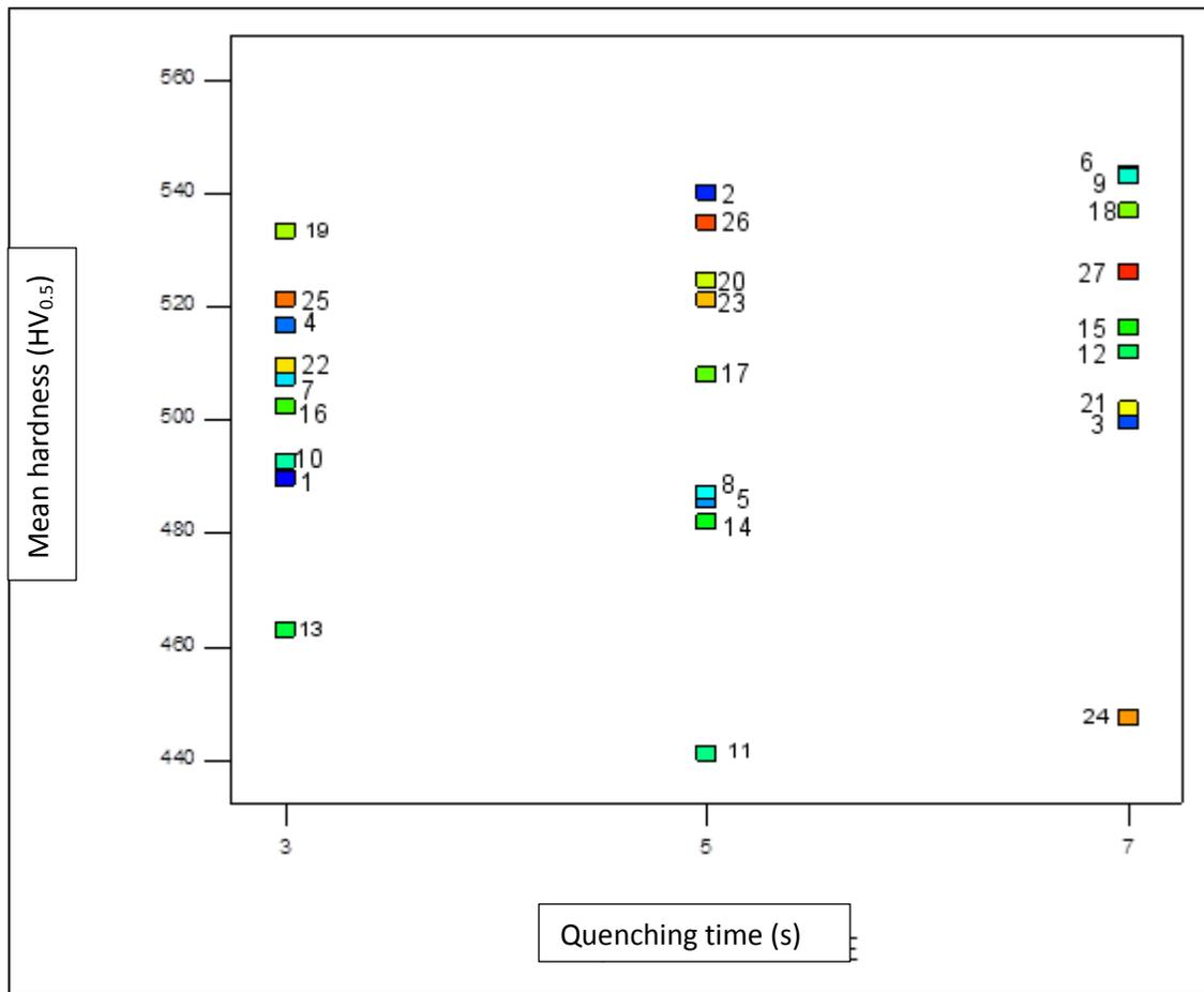
**Figure 4.3** Quenching time (s) VS hardness test (HV<sub>0.5</sub>)
