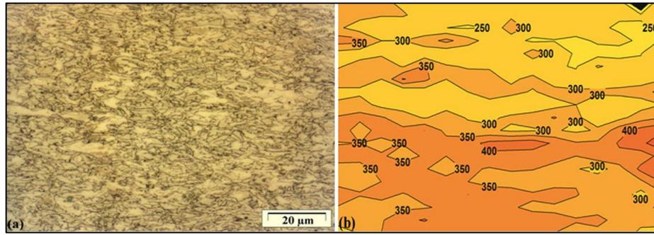
**Figure 2.10**(a) Microstructure and (b) hardness map of the specimen deformed at 650°C with strain rate of  $0.1 \text{ s}^{-1}$  [13].
