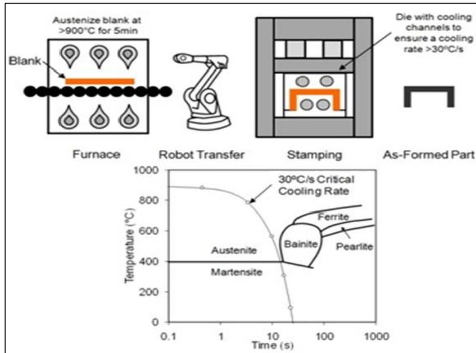
**Figure 2.2** The direct hot stamping method [5].
