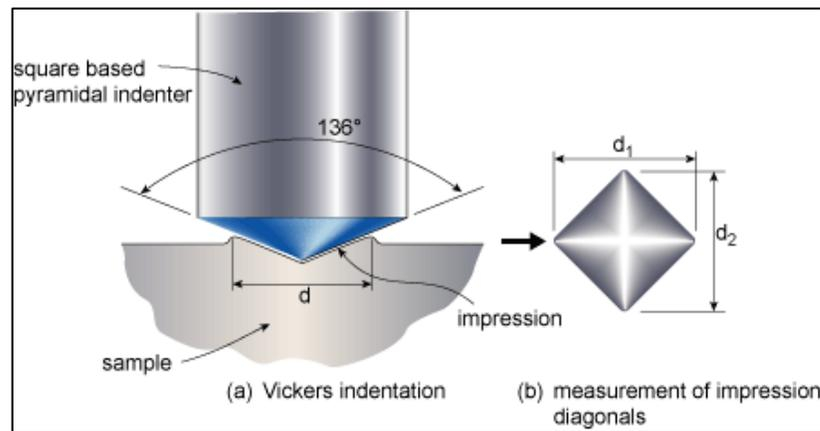
**Figure 3.8** Vickers indentation and measurement of impression diagonals.
