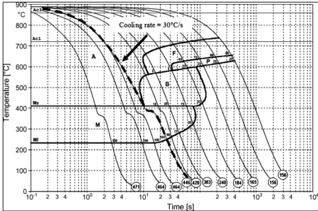
**Figure 2.6** Continuous cooling transformation diagrams [[7].
