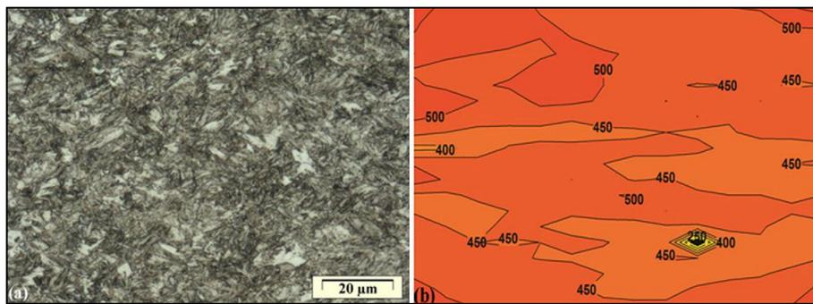
**Figure 2.9** (a) Microstructure and (b) hardness map of the specimen deformed at 900°C with strain rate of 1.0 s<sup>-1</sup> [13].
