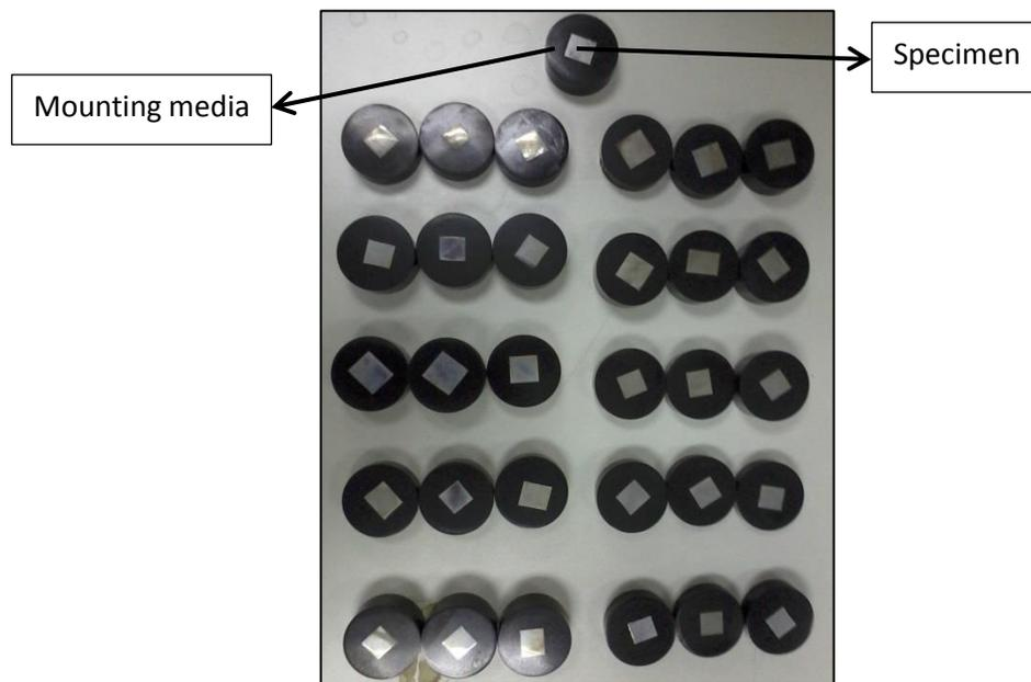
**Figure 3.7** Specimen preparations for testing
