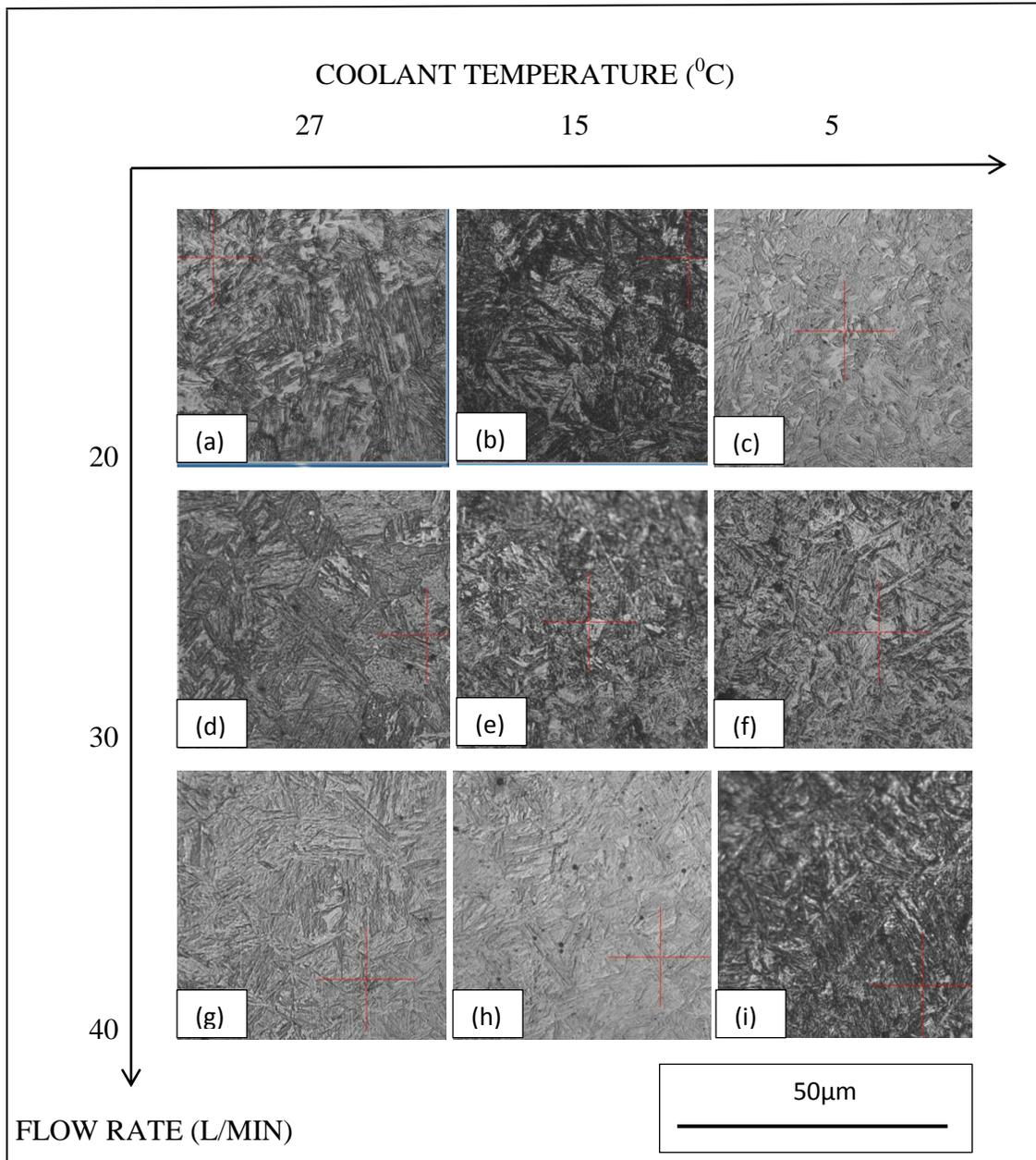
**Figure 4.8** Micrograph of martensite structure produced at different coolant temperature and flow rate of (a), (b), and (c) 20 L/min, (d), (e), and (f) 30L/min, and (g), (h), and (i) 40L/min.
