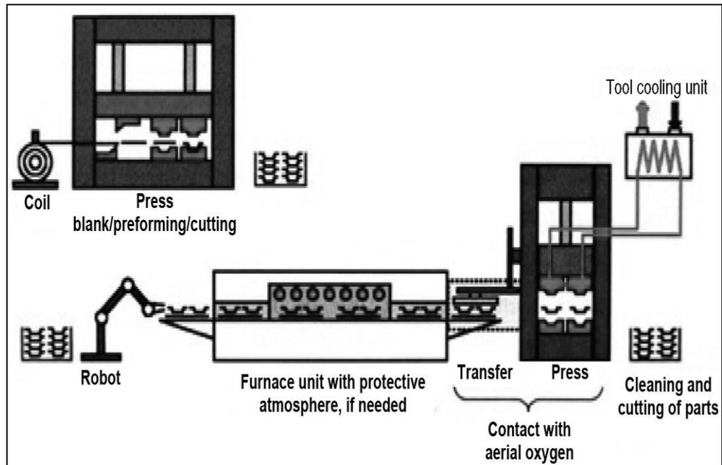
**Figure 2.3** The indirect hot stamping method [7].
