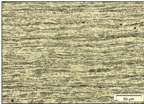
**Figure 2.7** Microstructure of the as-delivered 22MnB5 steel [15].
