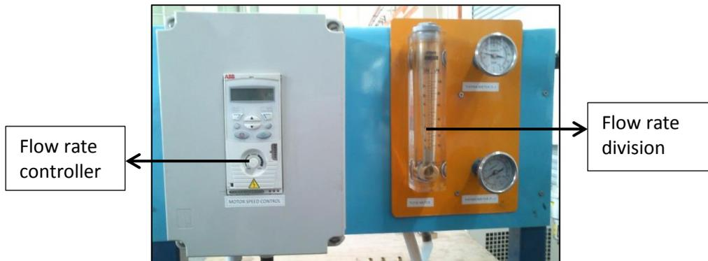
**Figure 3.6** Flow rate of the coolant
