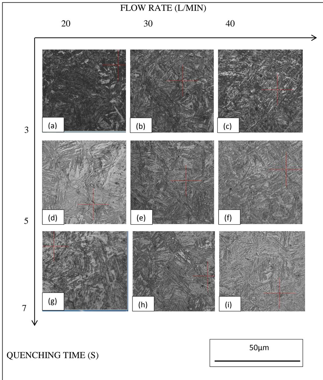
**Figure 4.6** Micrograph of martensite structure produced at different flow rate and quenching time of (a), (b), and (c) 3 second, (d), (e), and (f) 5 second, and (g), (h), and (i) 7 second.
