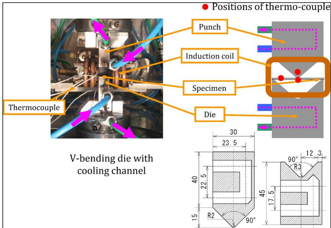
**Figure 2.5** Position of the thermocouple and die cooling channel [5].
