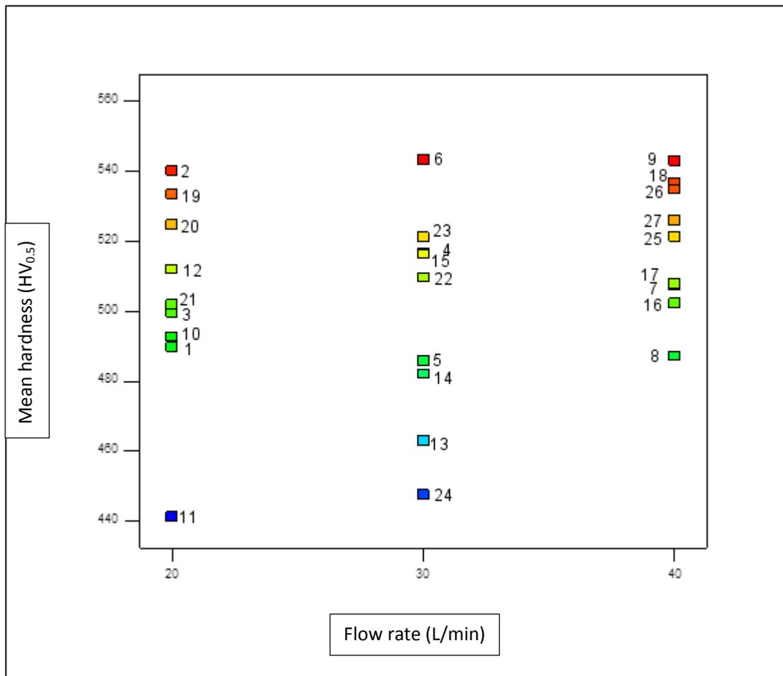
**Figure 4.4** Flow rate (L/min) VS hardness value (HV<sub>0.5</sub>)
