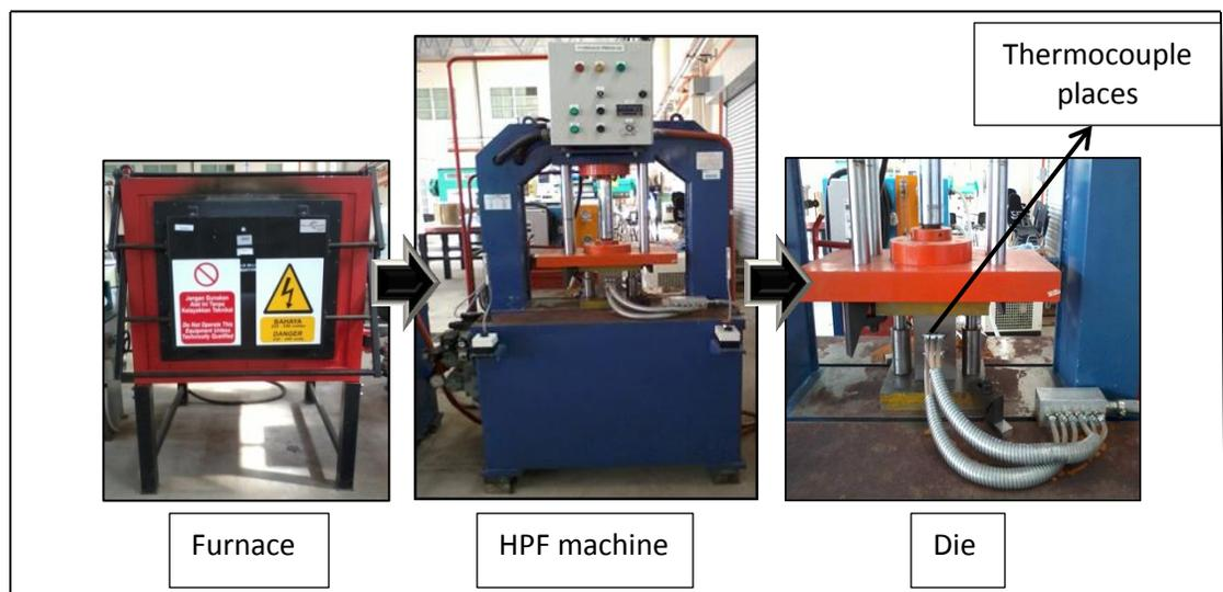
**Figure 3.3** Process of hot press forming.
