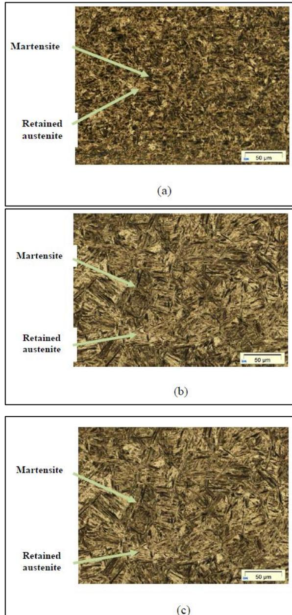
**Figure 2.8** Comparing the microstructures of 22MnB5 after austenitizing and quenching with, (a) the austenitization temperature of 900°C, (b) the austenitization temperature of 1100°C, and (c) the austenitization temperature of 1200°C [15].
