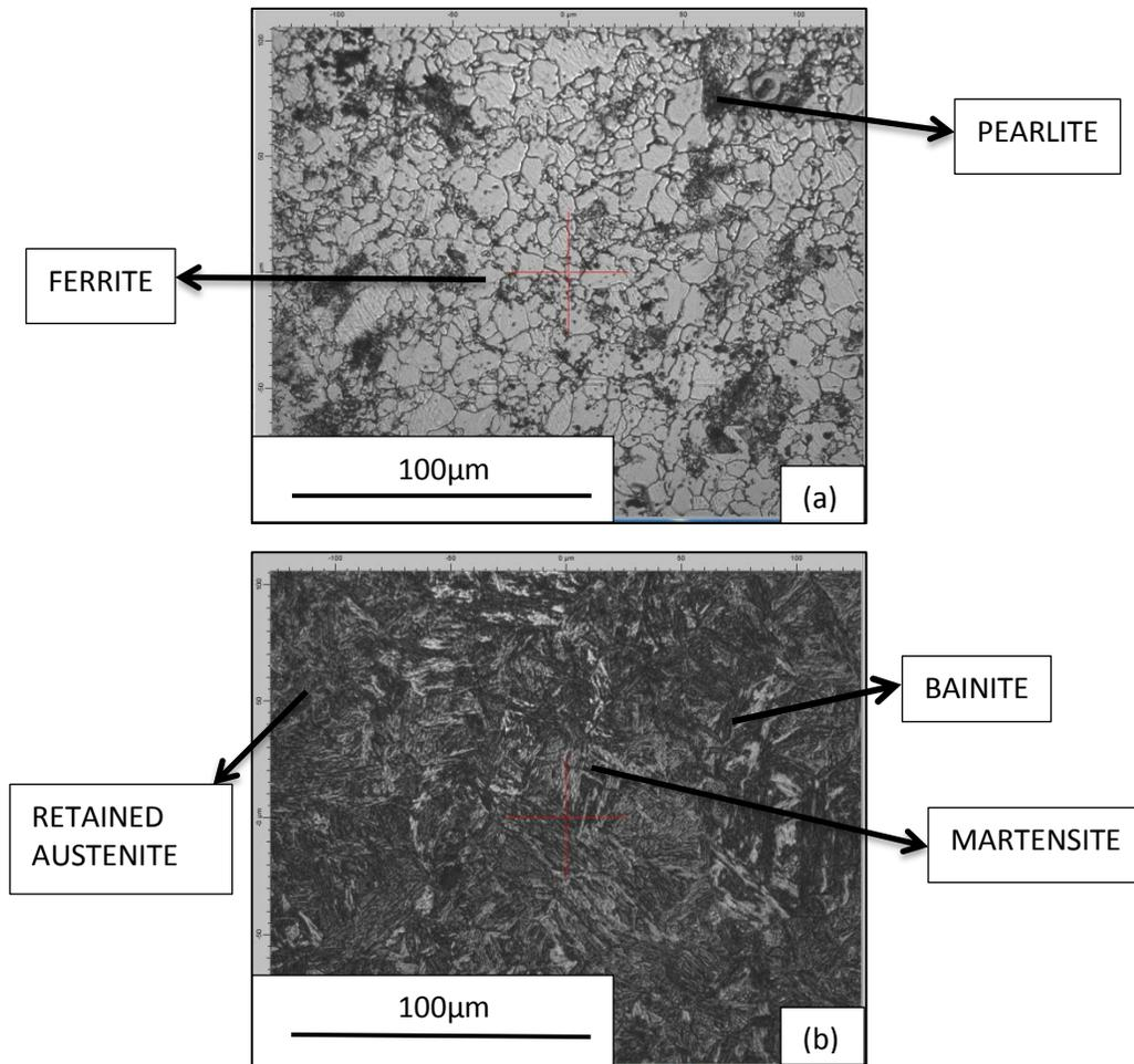
**Figure 4.1** Microstructure of the specimen before (a) and after (b) being hot stamped.
