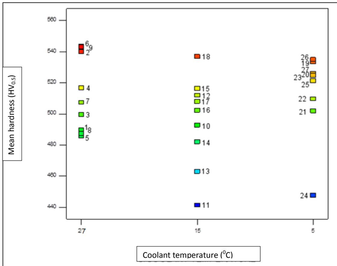
**Figure 4.5** Temperature of the coolant (°C) VS hardness value (HV<sub>0.5</sub>)
